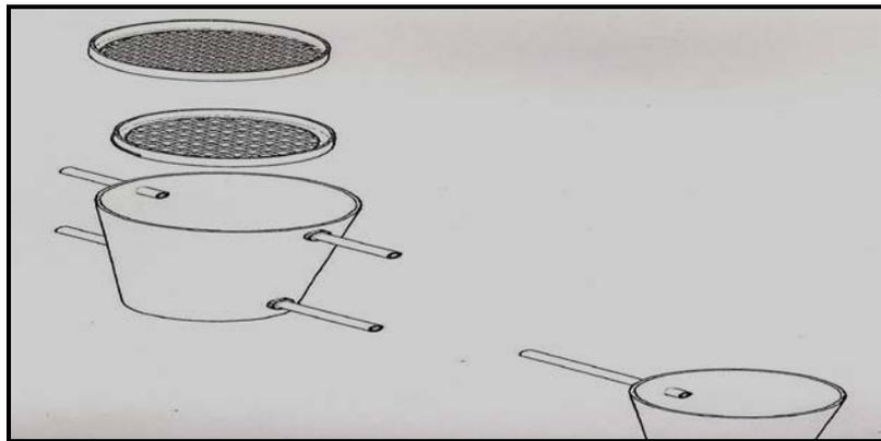
Figure 7. Assembly drawing showing the arrangement of filter elements of the plant
