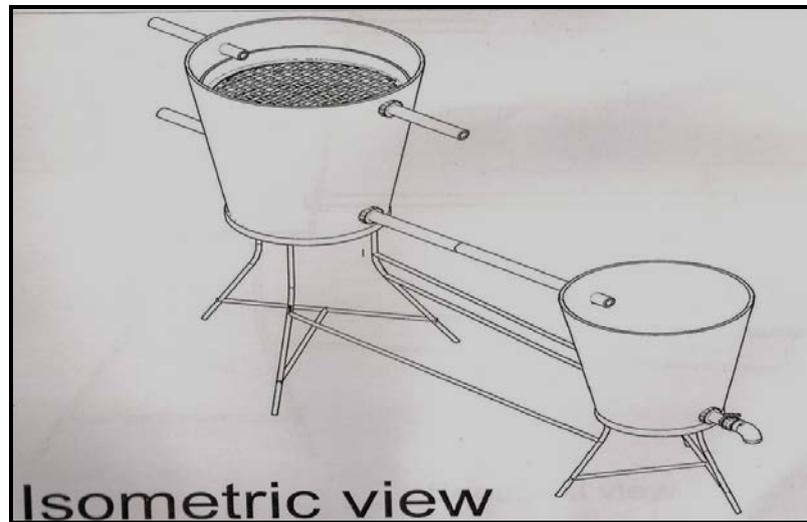
Figure 8. Isometric view of the filtration plant
