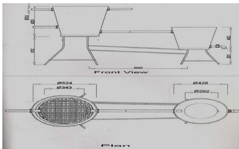
Figure 5. Orthographic plan and front views of the filtration plant
