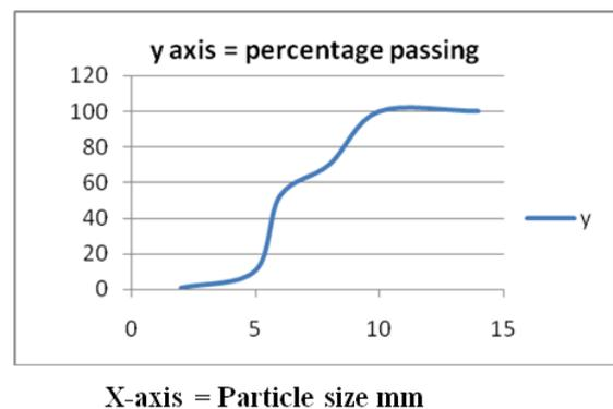
Figure 9. Specification for filter gravel 6-10 mm sieve analysis graph
