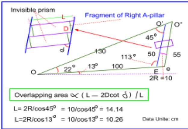
**Figure 8.** Illustration of calculations of the overlapping area between two invisible prisms
