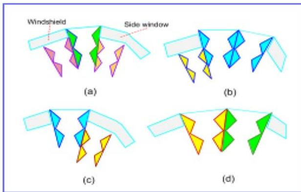
**Figure 9.** Various combinations of invisible prisms setting up A-pillars suitable to all sorts of vehicles
