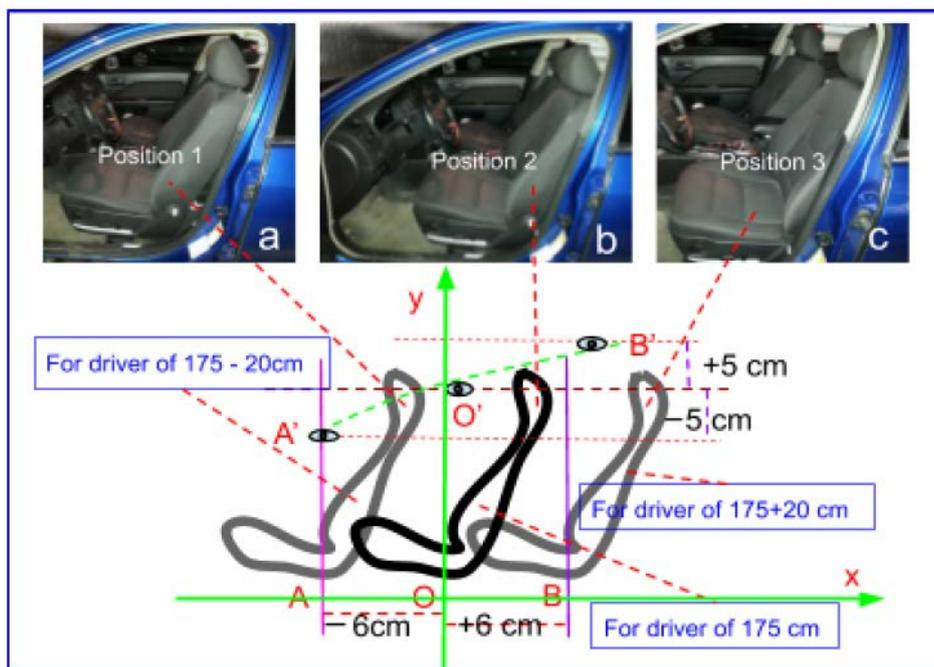
Figure 4. Positions of car seat for drivers of different stature
