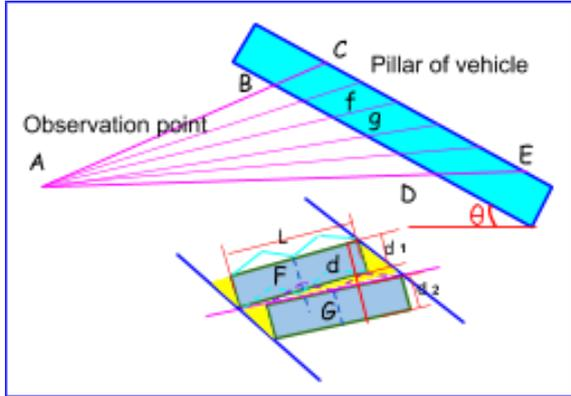
Figure 1. Illustration of the relative position between the pillar and observation point
