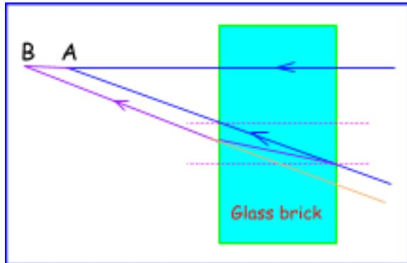
Figure 8. Refractive light path of Figure 7
