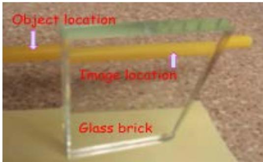
Figure 7. Glass chunk to refract light
