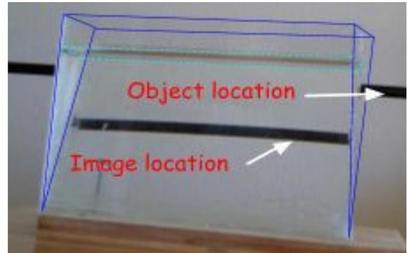
Figure 3. V-like triangular prism image formation
