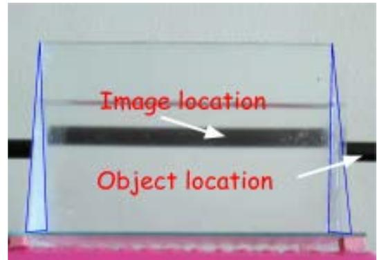
Figure 4. Δ-like triangular prism and image formation
