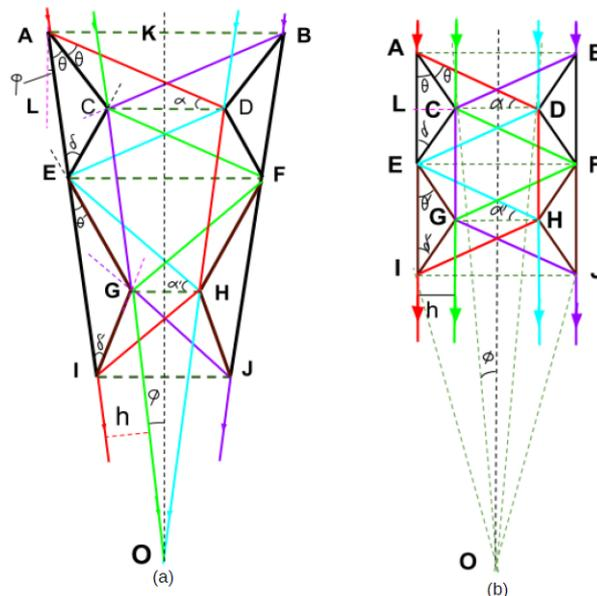
**Figure 12(a).** The illustration shows all the parameters necessary to determine the whole quadrangular prism of self-invisibility, (b) The illustration shows all the parameters necessary to determine the Extrapolation
