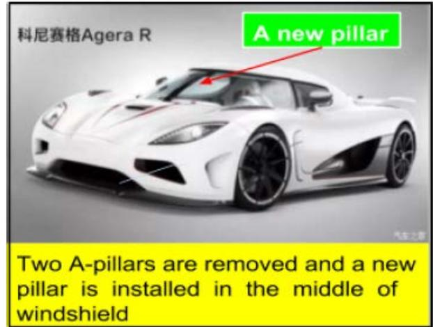
Figure 9. Car moving two A-pillars to middle of windshield
