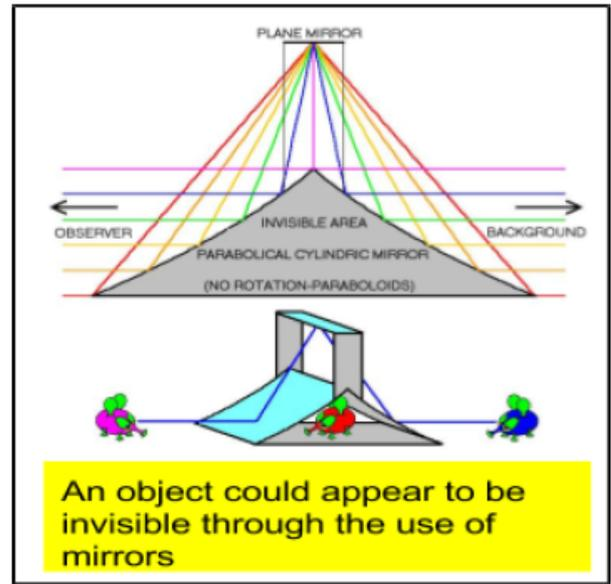
Figure 2. Illustration of parabolic mirrors for stealth
