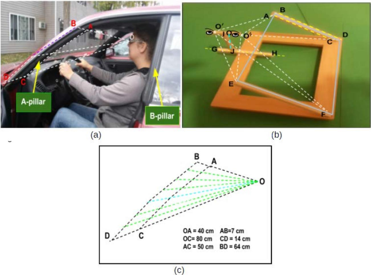
**Figure 13.** (a) Driver sitting in car, (b) Model of observer point and A-pillars, (c) Some parameters necessary obtained from observer point to A-pillar
