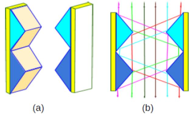
**Figure 11.** (a) When the distance between a pillar and an observer goes to infinity, the quadrangular prism converts into a rectangular prism and all the base triangles of the triangular prisms become isosceles triangles, (b) The light path of the lateral face mirrors of the isosceles triangular prisms
