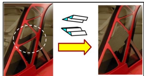
Figure 20. Making a use of quadrangular prism to lattice-like existing A pillar provides a better view field for drivers
