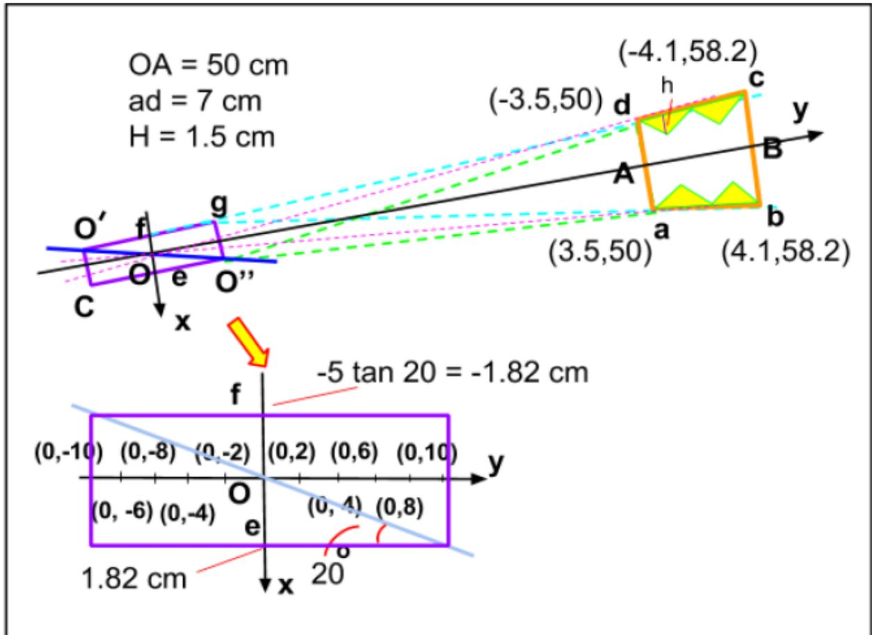
Figure 15. (a) Cross section of right A-pillar and the movement of observer's eye position
