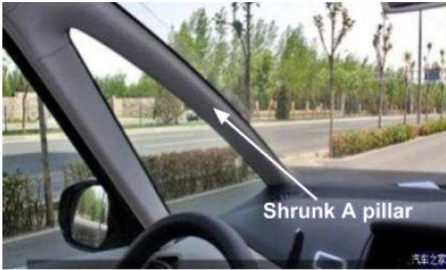
Figure 7. Triangular shape A-pillar of small size
