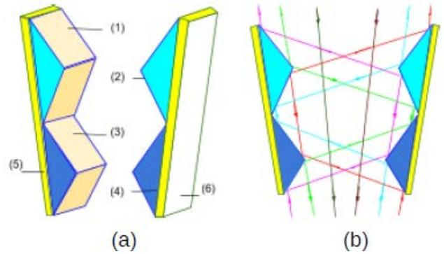
**Figure 10.** (a) Illustration of the quadrangular prism of self-invisibility (1) and (2) are two identical triangular prisms; (3) and (4) are also identical triangular prisms. (5) and (6) are identical transparent rectangular prisms, (b) The light path by relevant mirrors of lateral faces of all triangular prisms
