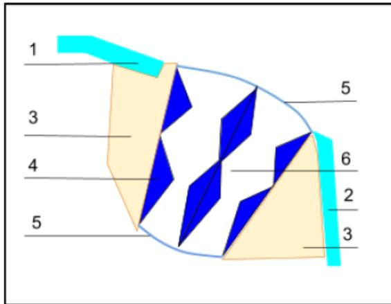
Figure 19. Illustration of an invisible quadrangular prism to replace the conventional right A-pillar of a vehicle, (1) windshield; (2) side window; (3) transparent cushions; (4) the quadrangular prism of self invisibility; (5) transparent covers; (6) transparent material
