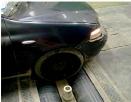
Figure 3. Overview of the vehicle on chassis dynamometer roller
