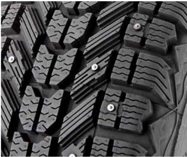
Figure 3. Example of studded tire type tread
