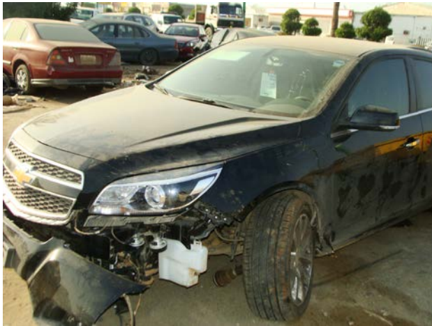
Figure 1. Single primary impact vehicle (Front) with secondary impact on opposite side
