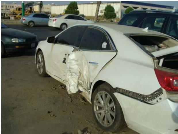
Figure 2. Primary impact on same side with secondary impact in front and back
