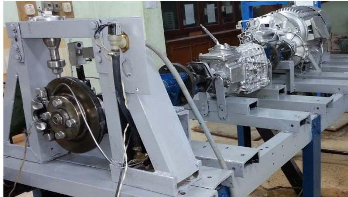
Figure 1. Main components of the brake dynamometer
