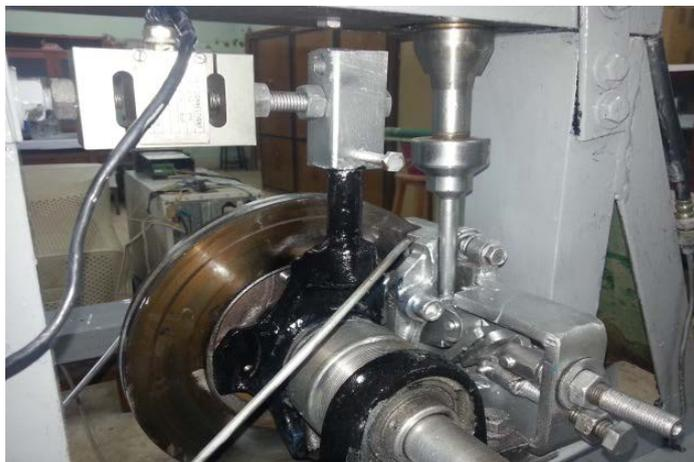
Figure 2. Modified (wedge) disc brake
