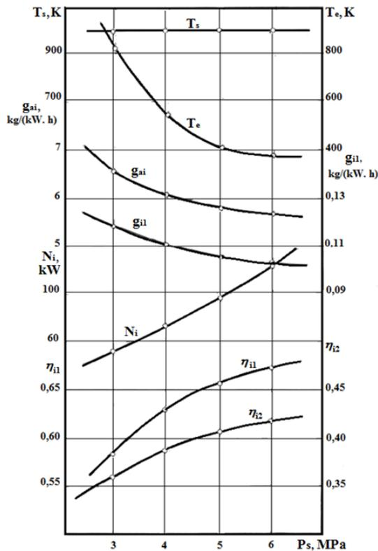
Figure 4. Influence of the pressure of combustion products  $p_s$  in the zone located above the piston on the indicated parameters of the external combustion engine at  $\alpha = 3$
