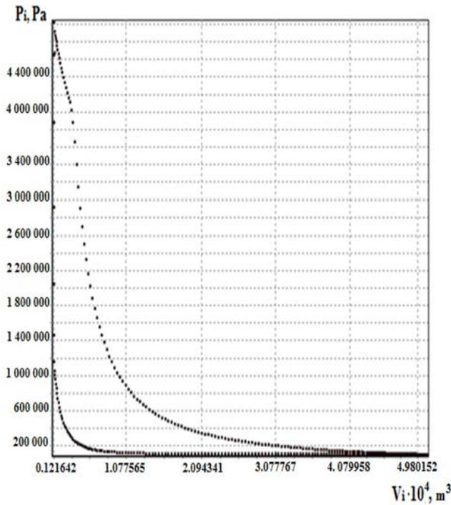
Figure 3. Cylinder pressure external combustion engine ( $n = 5000 \text{ min}^{-1}$ , air pressure in the zone-buffer  $p_s = 5 \text{ MPa}$  and the air to fuel ratio in the combustion chamber  $\alpha = 3$ )
