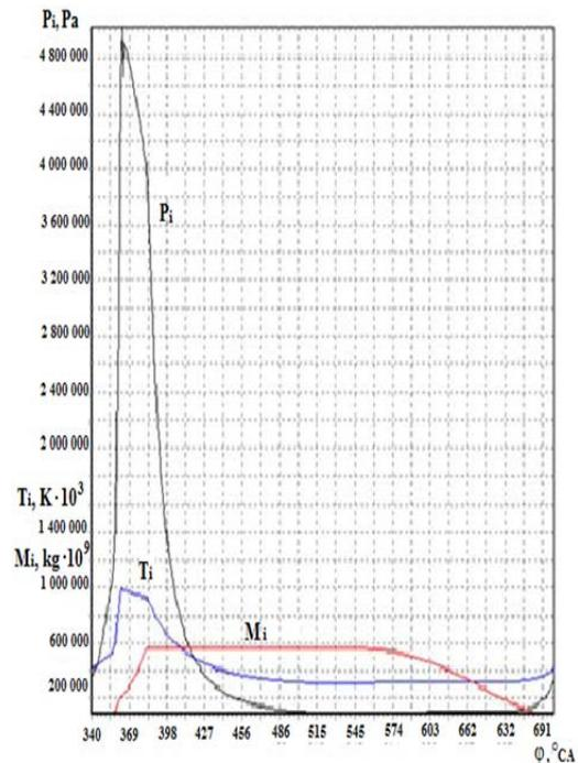
Figure 2. Variation in the charge parameters in the combustion chamber in the zone above the piston with crank angle
