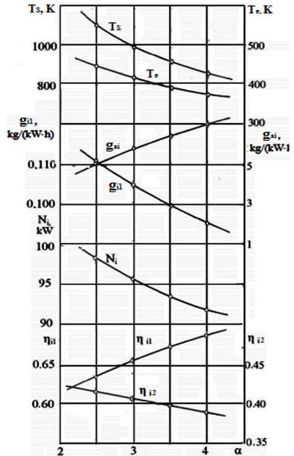
Figure 5. Influence of the variation of the air to fuel ratio  $\alpha$  in the combustion chamber, on the indicated parameters of the external combustion engine at  $p_s = 5 \text{ MPa}$
