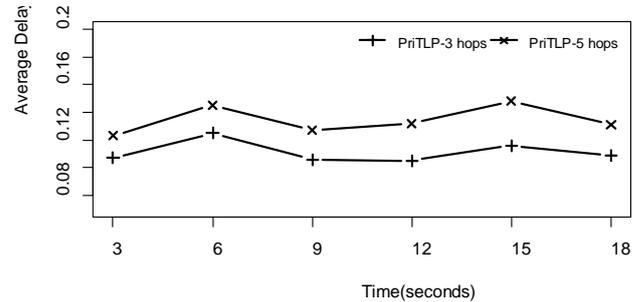
Figure 10. Analyzing an average delay using 6+1 RF nodes over 3 and 5 hop topology at different simulation time. Nodes are placed randomly
