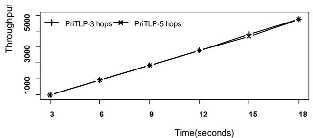
Figure 11. Analysis of average throughput over 6+1 RF nodes with 3 and 5 hop topology at different simulation time. The placement of nodes is random
