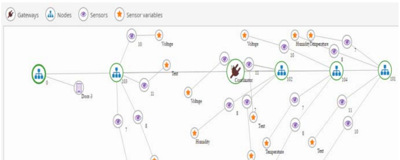
**Figure 3.** Screenshot of 3-hop node topology captured during run time experimentation in real time scenario using a cloud solution. Eye symbol and star symbol indicates sensing device logical id and sensing device type.
