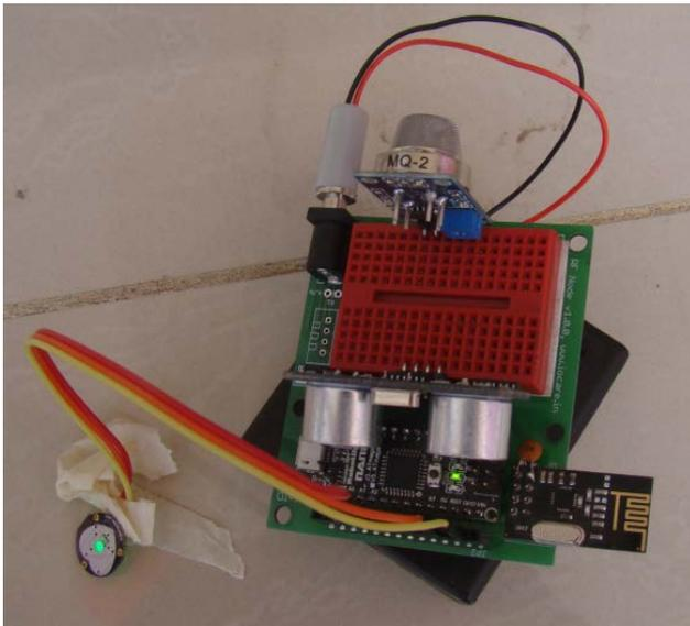
**Figure 2.** (RF Node) photograph shows the single node RF node view. A node is equipped with an additional breadboard for connecting the multiple sensing devices for achieving the different types of traffic in small size networks
