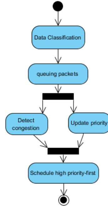
Figure 7. Operational flow of intermediate node over hop by hop topology
