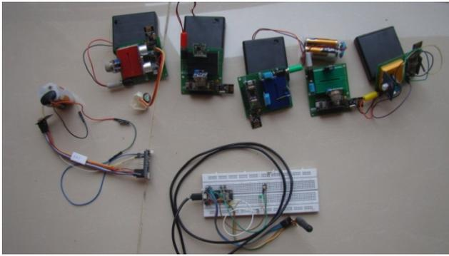
**Figure 1.** 6+1 RF TestBed Setup used in mesh based topology for heterogeneous wireless sensor networks. Over the breadboard, the coordinator is set up for controlling all source nodes
