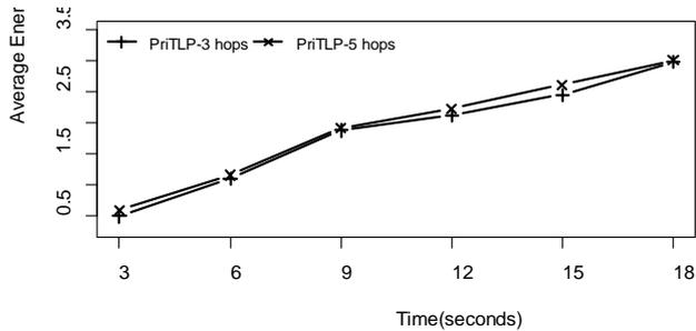
Figure 9. Analysis of average energy consumption over 6+1 RF nodes with 3 and 5 hop topology at different simulation time. The placement of sources is random
