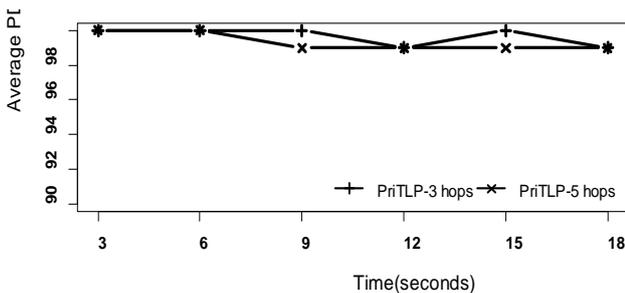
Figure 14. Analysis of average packet delivery ratio with variable hop count (0.05second interval time)
