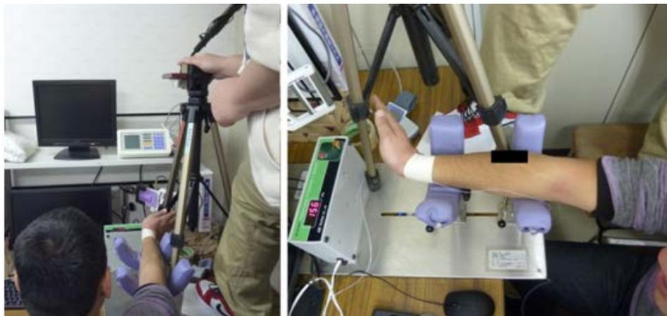
**Figure 4.** Measurement of (active) dorsal flexion angle using a digital camera with a leveler installed
