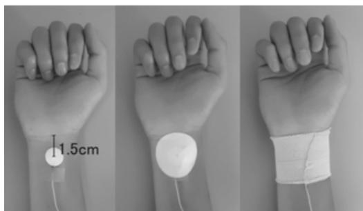
**Figure 4.** (a) only sensor, (b) sensor with cover tape, and (c) wrist taping with sensor and wrapped cover tape
