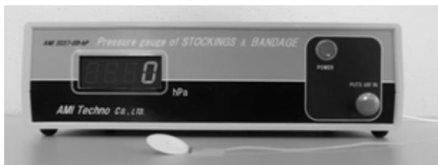
**Figure 2.** Pressure Measuring System for Stockings and Bandages (AMI3037-SB)
