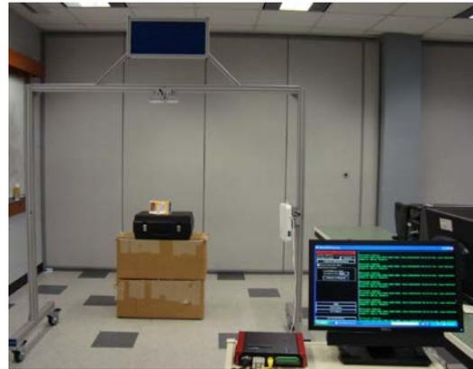
**Figure 2.** The BlueBean RFID Development Lab System
