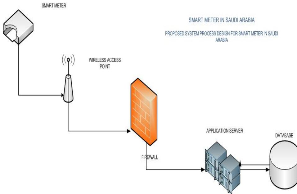
Figure 9. Proposed System Process Design for Smart Meter in Saudi Arabia
