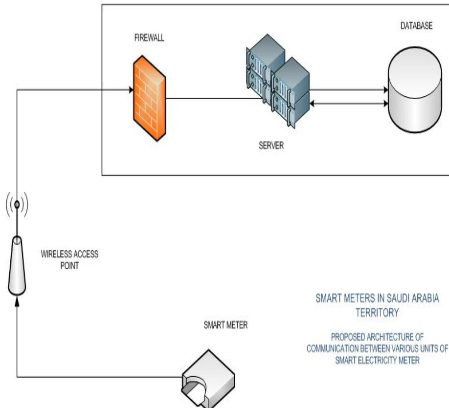
Figure 8. Proposed Architecture of Communication between various units of Smart Model
