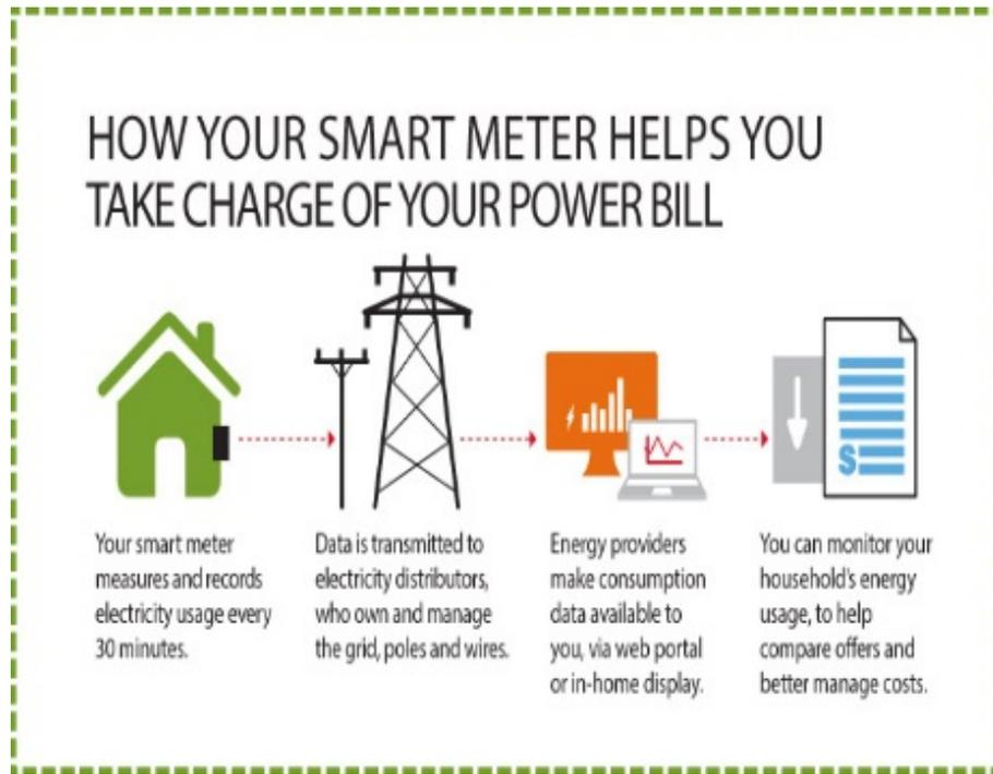
Figure 1. SMART METER LIFECYCLE [17]
