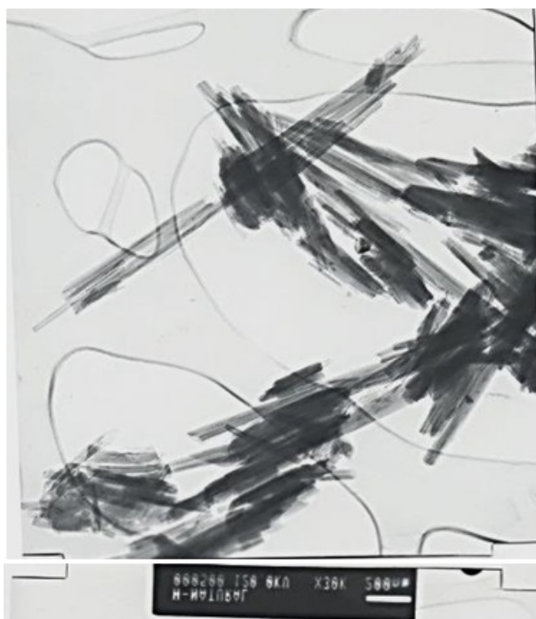
Figure 3. TEM micrographs of halloysite nanotubes (HNTs) studied
