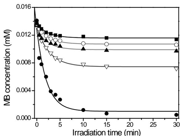
**Figure 3.** The degradation of MB concentration at different times of UV irradiation in the presence of  $\text{TiO}_2^c$  (●),  $\text{TiO}_2^{0.5}$  (▽),  $\text{TiO}_2^1$  (▲),  $\text{TiO}_2^2$  (○), and  $\text{TiO}_2^4$  (■) NPs catalysts. The lines are their respective best fitting with an exponential decay function
