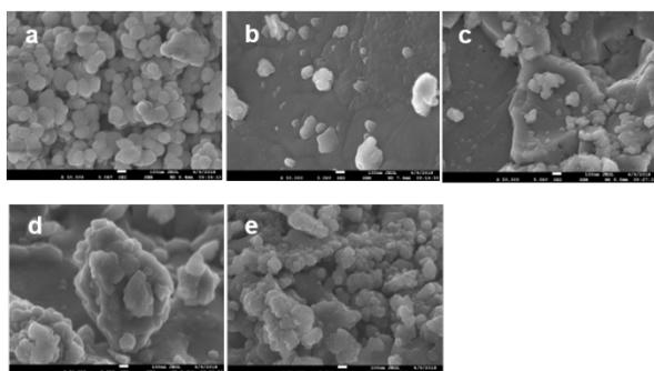
**Figure 1.** SEM images of  $\text{TiO}_2^c$  (a) along with  $\text{TiO}_2^{0.5}$  (b),  $\text{TiO}_2^1$  (c)  $\text{TiO}_2^2$  (d), and  $\text{TiO}_2^4$  (e). The scale bar in the images is of 100 nm
