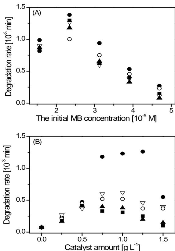
**Figure 4.** The effect of initial dye concentration (A) and catalyst dosage (B) on MB degradation in the presence of  $TiO_2^c$  (●),  $TiO_2^{0.5}$  (▽),  $TiO_2^1$  (▲),  $TiO_2^2$  (○), and  $TiO_2^4$  (■) NPs catalysts.
