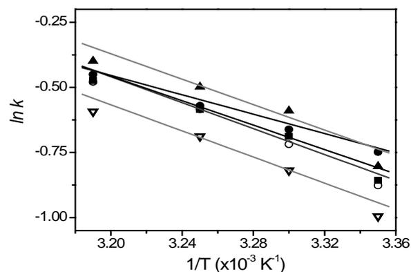
**Figure 5.** The plot of  $\ln k$  against inverse temperature,  $1/T$ , of the photocatalytic degradation of MB in the presence of  $TiO_2^c$  (●),  $TiO_2^{0.5}$  (▽),  $TiO_2^1$  (▲),  $TiO_2^2$  (○), and  $TiO_2^4$  (■) NPs catalysts. The straight lines are their respective best fit
