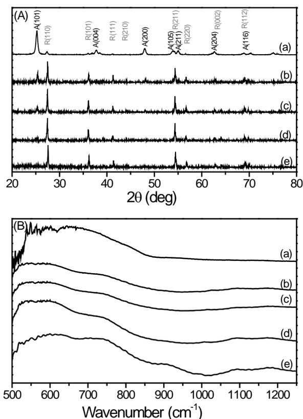
**Figure 2.** XRD pattern (A) and FTIR spectrum (B) of  $\text{TiO}_2^c$  (a),  $\text{TiO}_2^{0.5}$  (b),  $\text{TiO}_2^1$  (c),  $\text{TiO}_2^2$  (d), and  $\text{TiO}_2^4$  (e)
