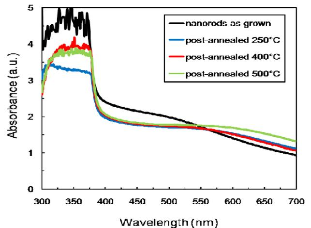
**Figure 11.** UV-vis absorbance spectra of ZnO nanorods [61]
