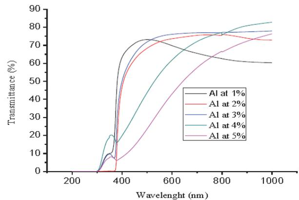
**Figure 19.** Transmittance spectra of ZnO nanorods for 1% to 5% doping [64]
