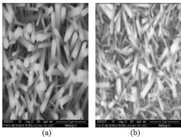
**Figure 12.** FESEM images of ZnO nanorods prepared using growth precursor with a concentration of (a) 0.02 M (b) 0.06 M [62]
