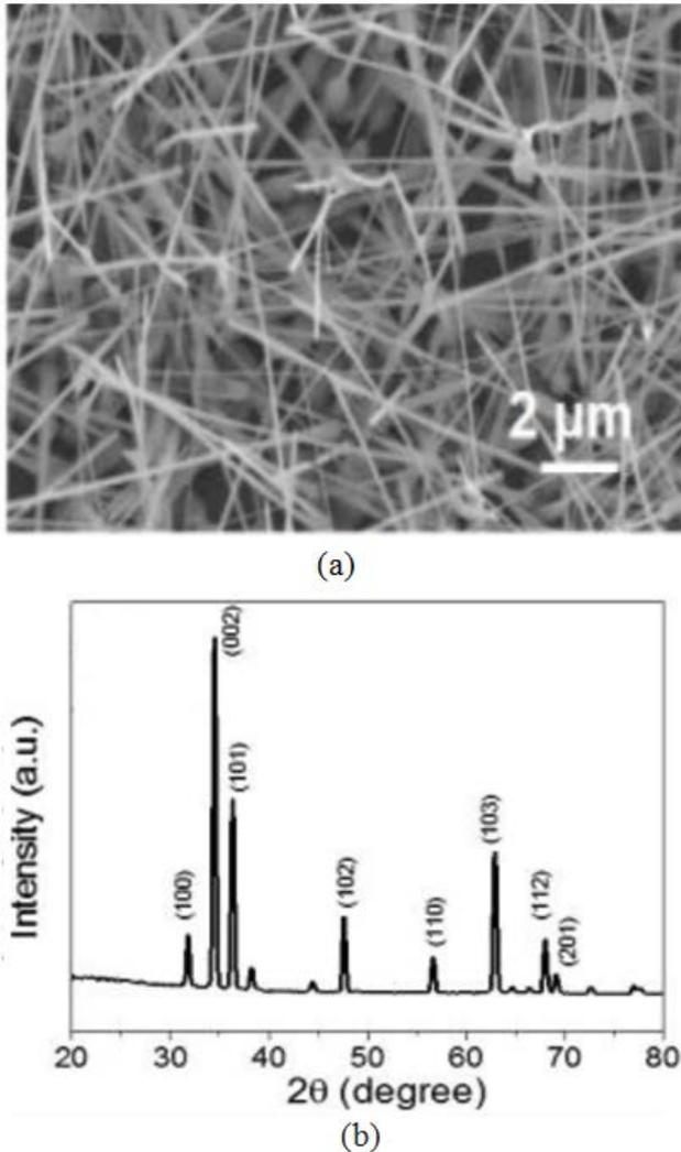
Figure 3. (a) SEM image of as-grown nanowires (b) XRD [47]
