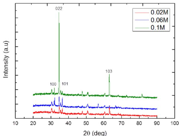
**Figure 13.** XRD pattern of ZnO nanorods prepared using growth precursor with a concentration of 0.02 M, 0.06 M and 0.1 M [62]
