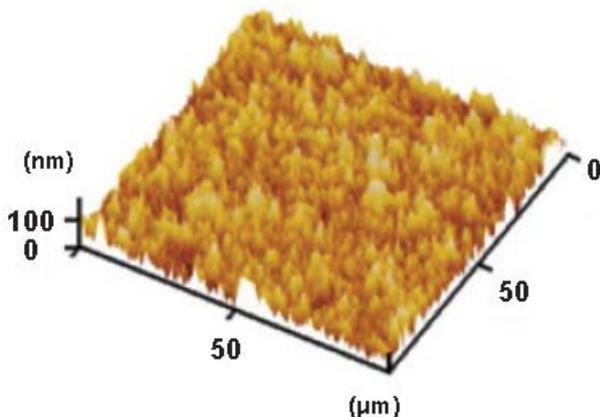
**Figure 9.** AFM images of ZnO seed layers [60]
