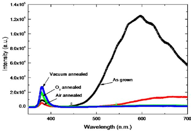
**Figure 16.** Room temperature PL of as-grown ZnO nanorods and annealed in various conditions [63]
