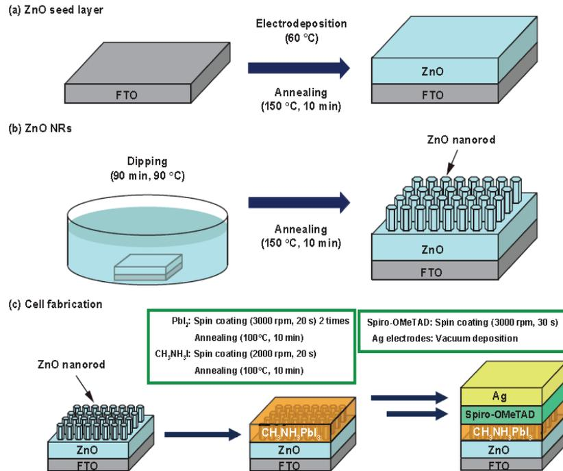
**Figure 8.** Schematic illustrations of fabrication processes of (a) ZnO seed layer, (b) ZnO nanorods, (c) ZnO nanorods/CH<sub>3</sub>NH<sub>3</sub>PbI<sub>3</sub> SC [60]
