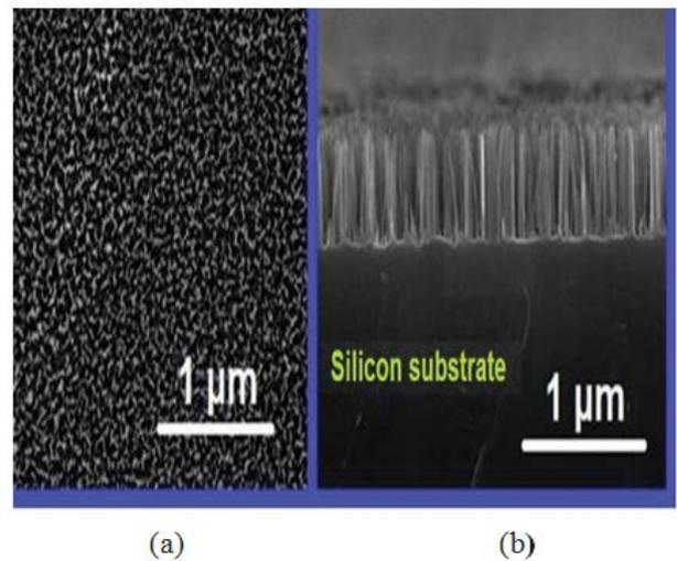
Figure 5. Top-view (a) and cross-sectional (b) FESEM image of bare Si nanowires [50]
