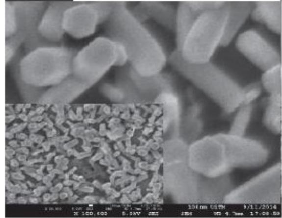
**Figure 17.** SEM of ZnO nanorods [64]
