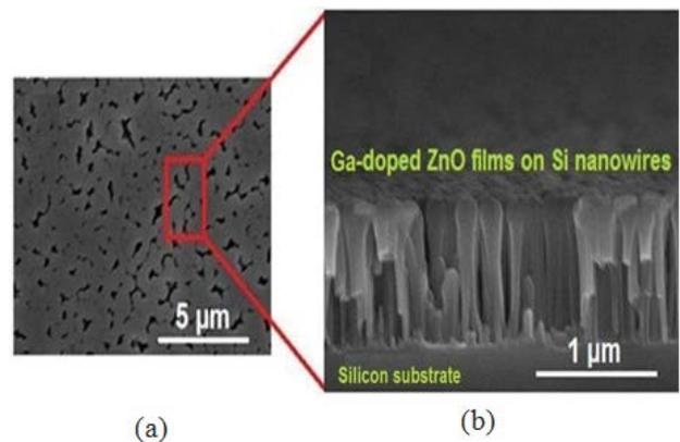
Figure 6. (a) Top-view (b) cross-sectional FESEM image of Ga-doped ZnO thin film coated onto Si nanowire arrays [50]
