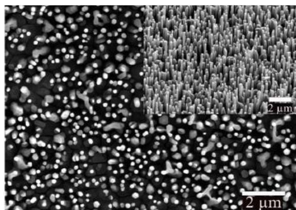
Figure 2. SEM image of as-grown ZnO nanowires [47]
