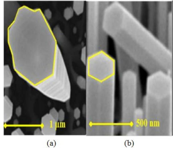
Figure 4. SEM images of ZnO nanowires: (a) undoped (b) doped [48]
