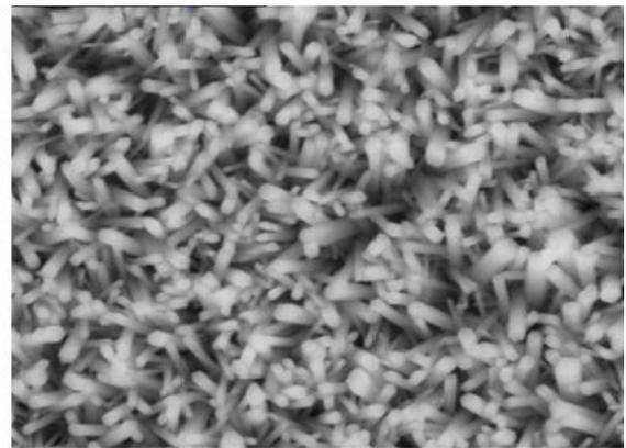
**Figure 10.** SEM images of as-grown ZnO nanorods layers [61]
