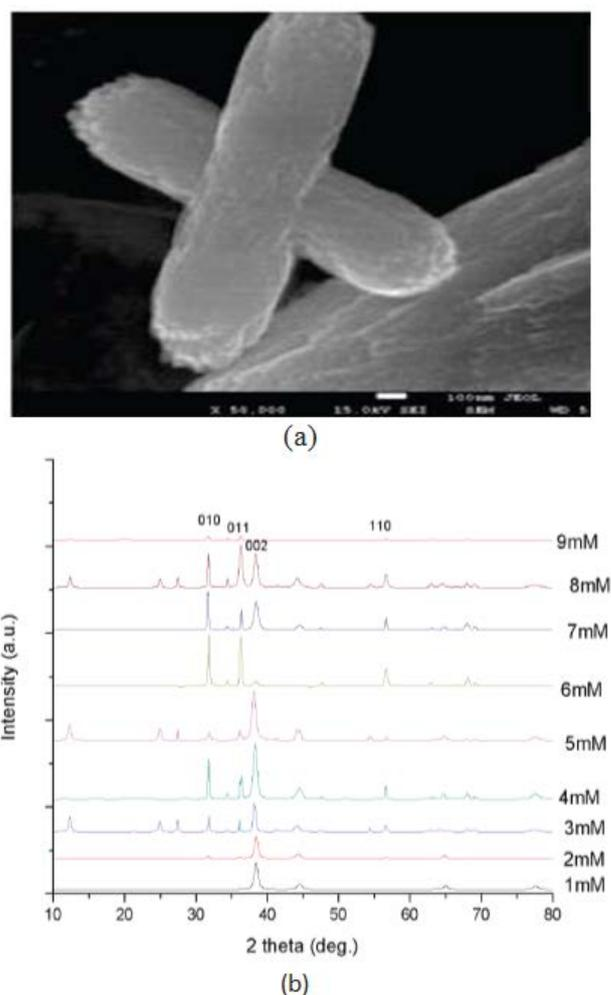
**Figure 7.** (a) SEM for ZnO nanorods [59], (b) XRD patterns of ZnO nanorods formed Cr-Au coated glass at different concentrations [59]
