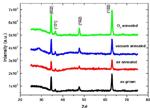
**Figure 15.** XRD spectra of as-grown ZnO nanorods and annealed in various ambient [63]
