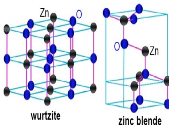
Figure 1. ZnO wurtzite structure [3]
