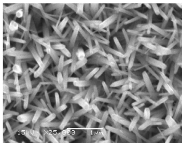
**Figure 14.** SEM of ZnO nanorods [63]
