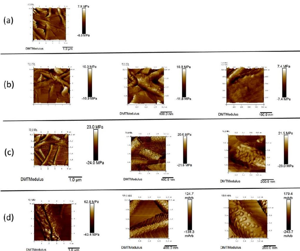
**Figure 2.** AFM DMT modulus images. High magnification DMT modulus images of the fiber surface clearly shows morphological appearance of the two, Ag and ZnO nanoparticles in micrograph. (a) Non-coated background fiber mat; (b) 30:30 (Ag:ZnO) sputtered fiber mat; (c) 100:30 (Ag:ZnO) sputtered fiber mat; (d) 30:100 (Ag:ZnO) sputtered fiber mat
