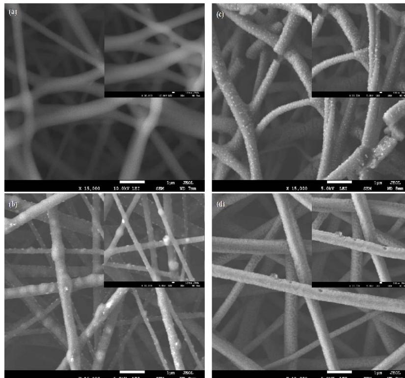
Figure 4. Scanning Electron Microscope (SEM) images for the nanofibers scaffold, (a) is the non-coated scaffold (negative control), (b) scaffold coated with 30:30 Ag:ZnO, (c) scaffold coated with 100:30 Ag:ZnO and (d) scaffold coated with 30:100 Ag:ZnO
