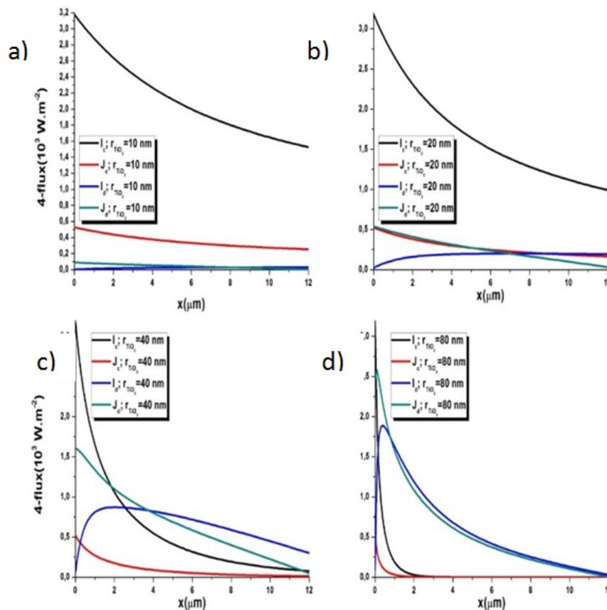
Figure 6. Collimated flux ( $I_c$ ,  $J_c$ ) and diffuse flux ( $I_d$ ,  $J_d$ ), for different radii of  $\text{TiO}_2$  (a – 10nm, b – 20nm, c – 40nm, d- 80nm) particle  $I_0=1000 \text{ W m}^{-2}$
