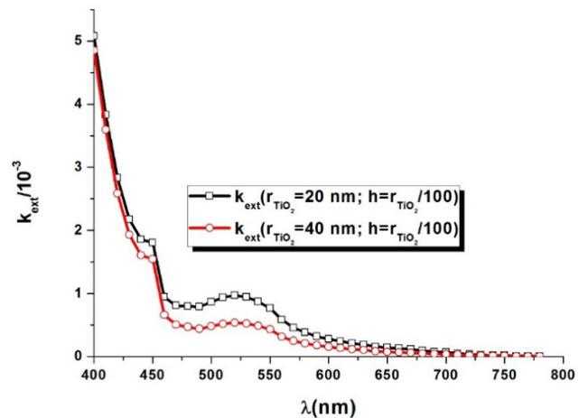
Figure 5. Extinction coefficient of photo-active layer (mixture  $TiO_2 + Z907+acetonitrile-I/I_3^-$ ) as a function of wavelength for different radii of the  $TiO_2$  particle
