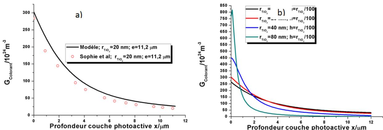
Figure 7. Generation rate of photo active layer as a function of the cell depth (a: comparison between our model and Sophie Wenger results, b: for different radii of  $\text{TiO}_2$ )
