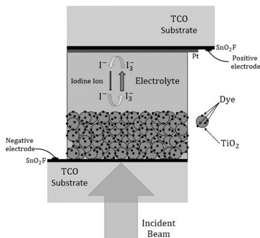
Figure 1. Structure of the Dye sensitized solar cell
