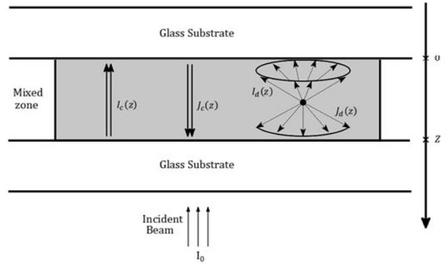
Figure 3. Schema of the cell with different flux
