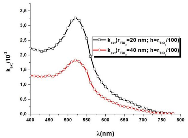
Figure 4. Extinction coefficient of photo-active layer (mixture  $TiO_2 + Z907$ ) as a function of wavelength for different radii of the  $TiO_2$  particle
