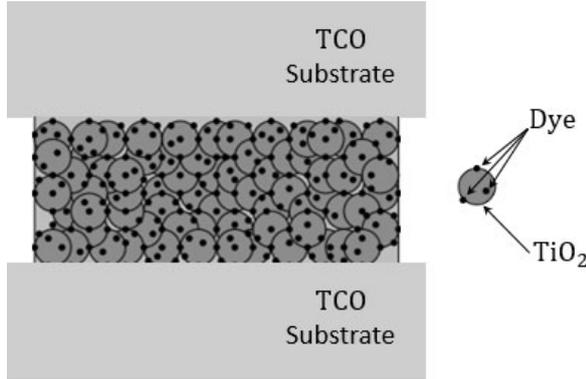
Figure 2. Schematic of the cell
