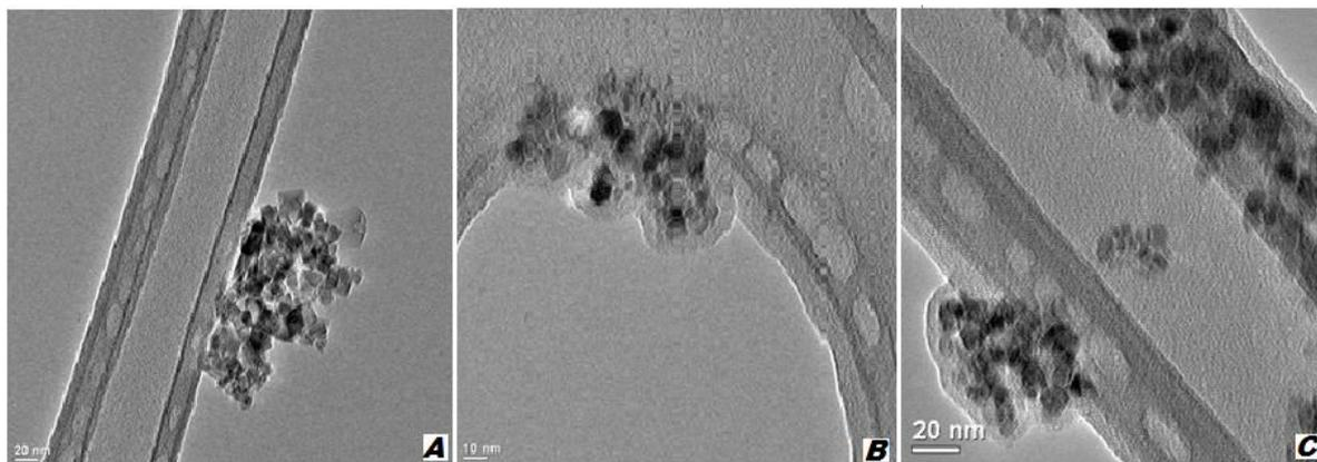
**Figure 1.** TEM images of the prepared MNP under very high resolution A-MNP, B-MNP@Cholesterol and C-MNP@Sulphadiazine
