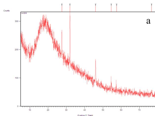
**Figure 2.** XRD patterns of silver nanoparticles synthesized from flower extract of *Ipomoea indica* treating with 1mM silver nitrate
