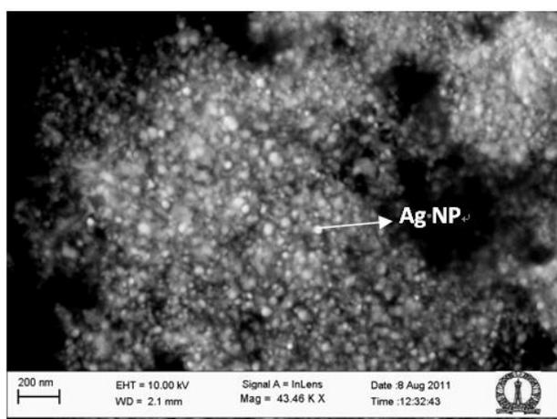
**Figure 3.** Scanning Electron Microscope image of silver nanoparticles (AgNP) synthesized from flower extract of *Ipomoea indica* treating with 1mM silver nitrate
