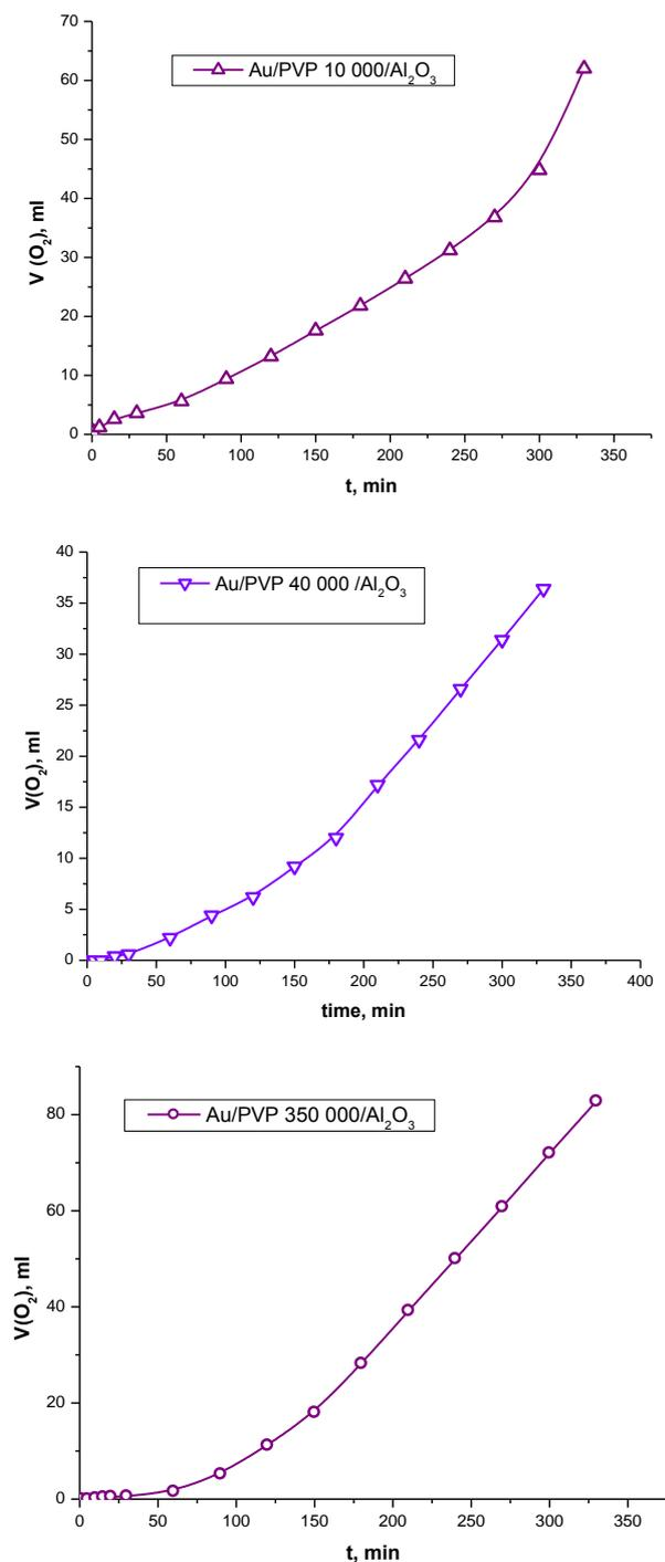
**Figure 5.** Time dependent decomposition of hydrogen peroxide in the presence of gold nanocatalysts
