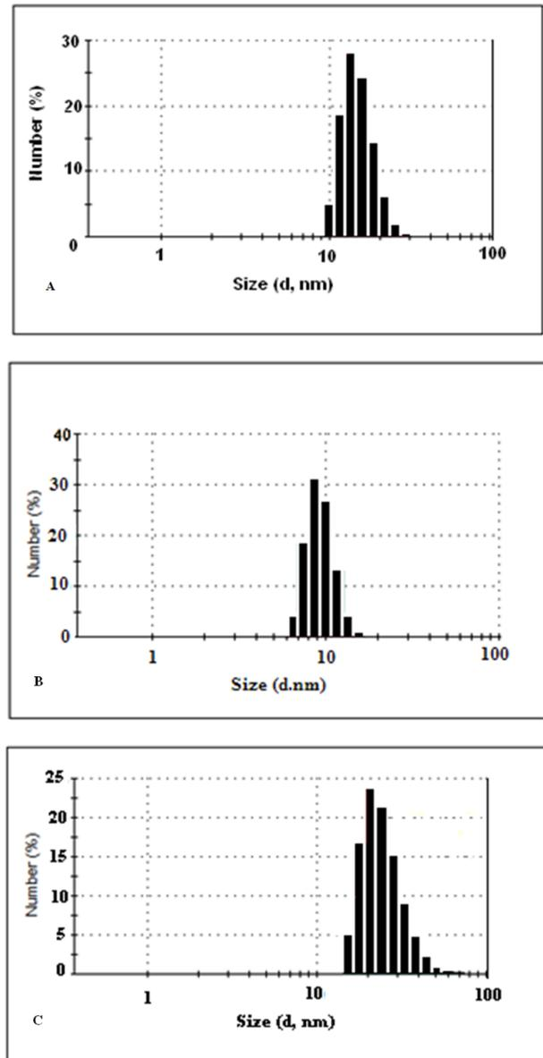
**Figure 3.** Size distribution of AuNPs stabilized by PVP with  $M_n = 10 \cdot 10^3$  (A)  $40 \cdot 10^3$  (B) and  $350 \cdot 10^3$  (C)
