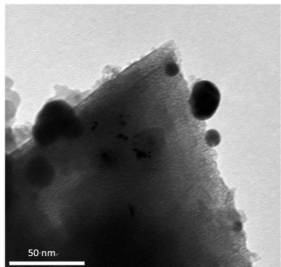
**Figure 4.** TEM image of AuNPs-PVP- $40 \cdot 10^3$  supported on  $\text{Al}_2\text{O}_3$
