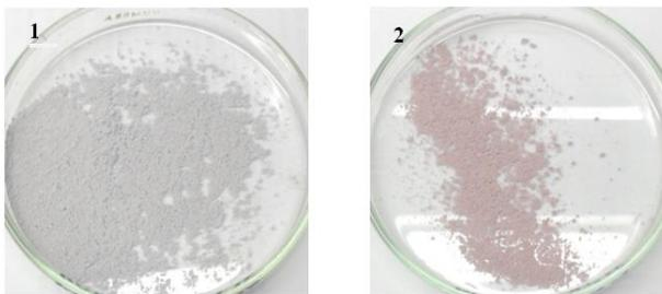
**Figure 2.** Samples of  $\text{Al}_2\text{O}_3$  with immobilized PVP-AuNPs.  $M_n = 40 \cdot 10^3$  (1) and  $350 \cdot 10^3$  (2)
