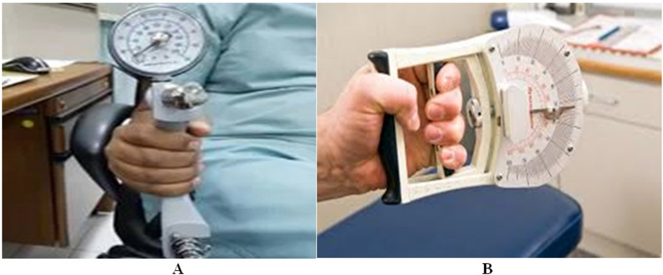
Figure 3. Assessment of muscle strength with a handgrip dynamometer (A) and handheld dynamometry [20]
