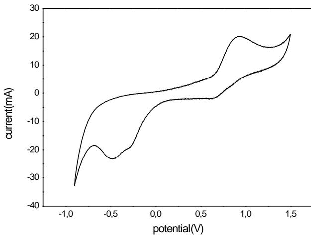
**Figure 5.** Cyclic voltammogram of *Rauwolfia v.* dye in acetonitrile solution containing 0.1 M TBATFB supporting electrolyte at 50 mV/s rate
