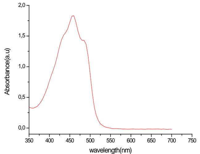
Figure 3. Absorption spectrum of Rauvolfia v. dye
