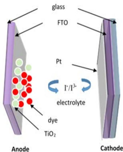
Figure 1. Diagram of dye sensitized solar cell components
