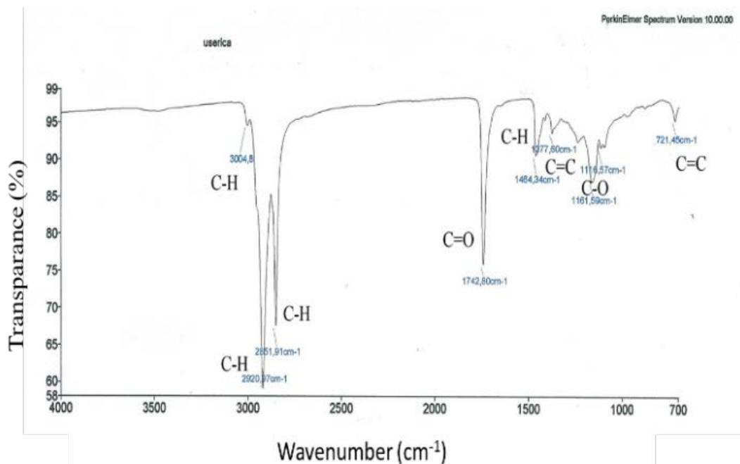
Figure 4. FTIR spectrum of Rauvolfia v. dye
