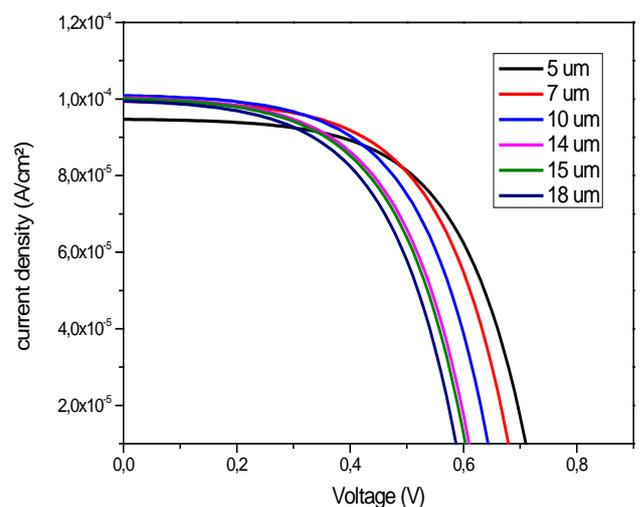
**Figure 6.** I-V characteristic of different  $TiO_2$  films
