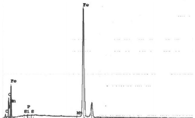
Figure 6. EDS spectrum of Bassar forged steel (BFS)
