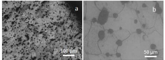
Figure 5. Optical micrographs of forged steel and chemical attacked sample
