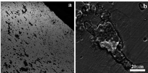
Figure 9. SEM micrographs of BFS, overview of the edge towards the inside (a), detail of a precipitate (b)
