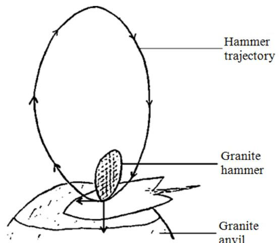
**Figure 2.** Kabiye forging technique
