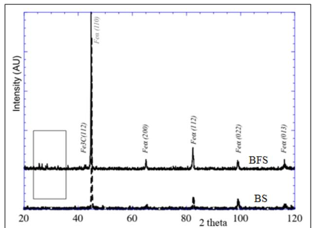
Figure 7. X-rays diffraction patterns of Bassar Forged Steel (BFS) and BS
