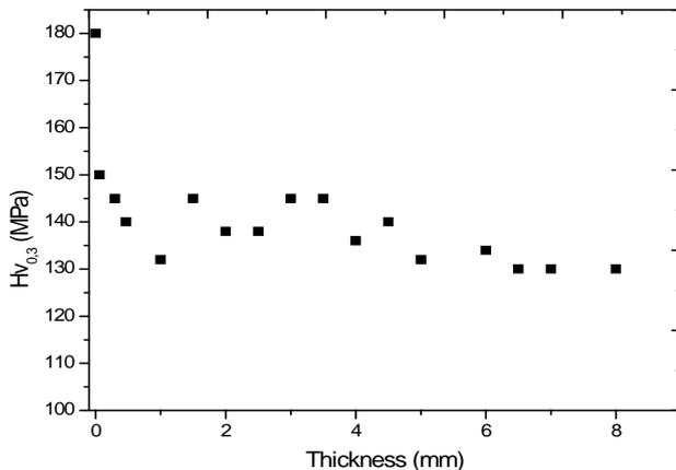
Figure 8. Vickers micro-hardness of BFS in function of its thickness
