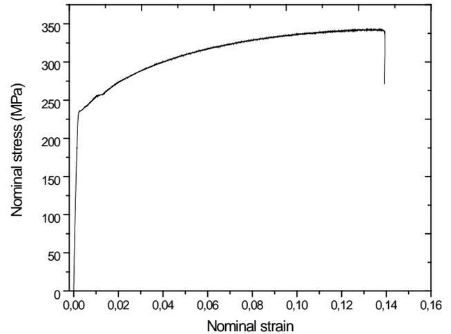
Figure 10. Nominal stress-strain curve of BFS
