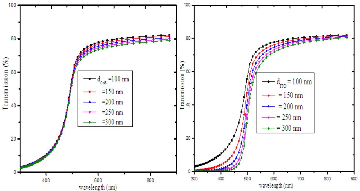
**Figure 5.** Variation of the transmission of the  $\text{Ta}_2\text{O}_5/\text{CdS}$  solar cell
