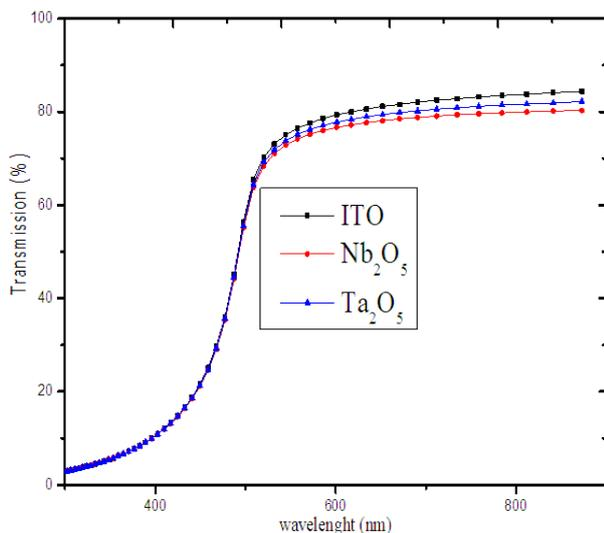
**Figure 6.** Variation of TCO/CdS solar cell transmission as a function of wavelength
