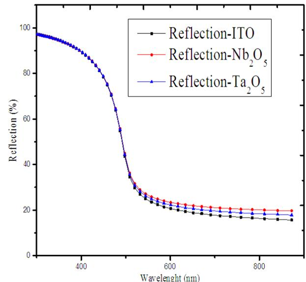
**Figure 7b.** Variation of the reflection of the CdS/CdTe thin film solar cell at 100 nm as a function of the wavelength
