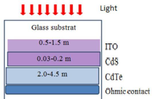
Figure 1. Classic CdTe cell prototype [5]
