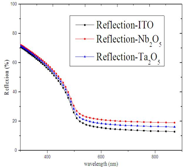
**Figure 7a.** Variation of the reflection of the CdS/CdTe thin film solar cell at 30 nm as a function of the wavelength
