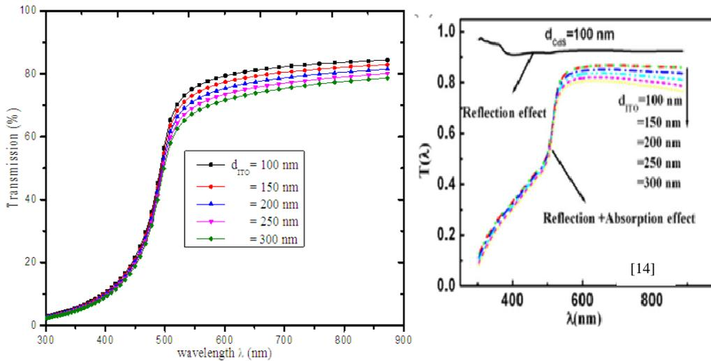
Figure 2. Variation of the glass/ITO/CdS solar cell transmission as a function of the wavelength (fixed CdS thickness)
