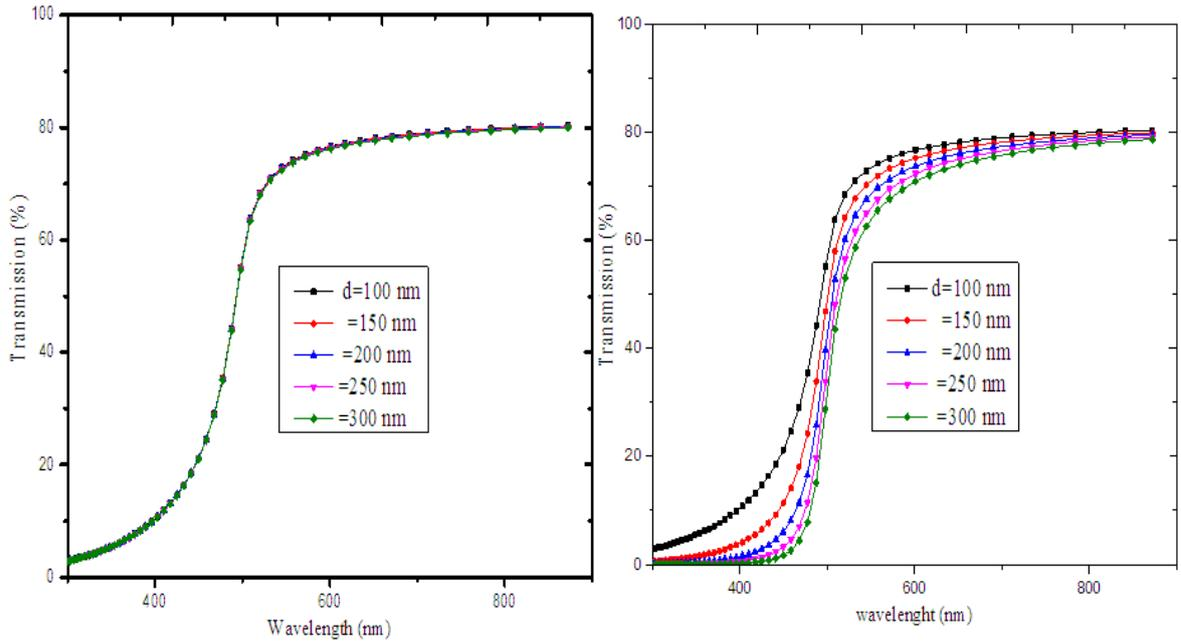
**Figure 4.** Variation of the transmission of the  $\text{Nb}_2\text{O}_5/\text{CdS}$  solar cell as a function of the wavelength
