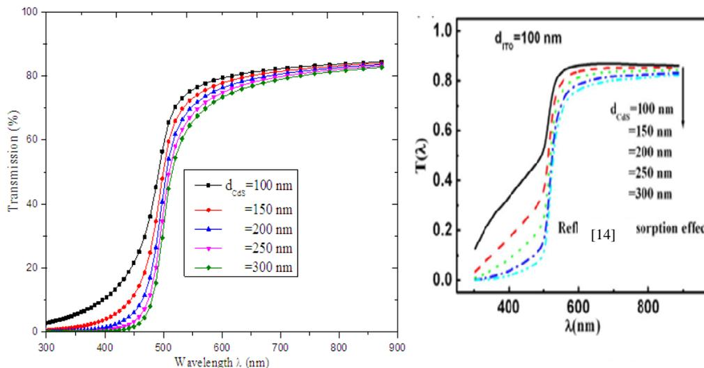
Figure 3. Variation Transmission photo cell glass/ITO/CdS versus the wavelength fixed ITO
