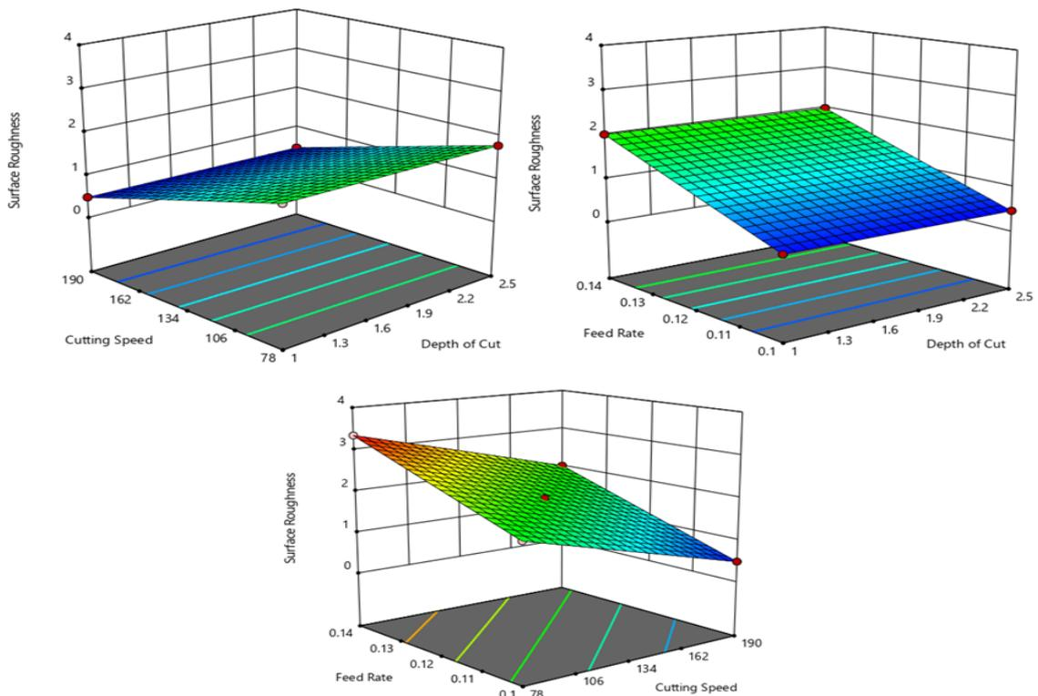
**Figure 3.** 3D surface plot of surface roughness with respect to cutting speed and depth of cut, with respect to feed rate and depth of cut and with respect to feed rate and cutting speed
