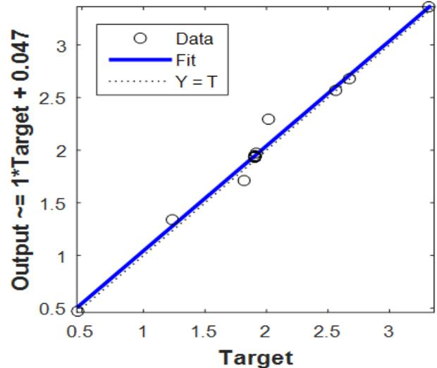
**Figure 4.** Linear Regressions plot for Experimental values of surface roughness ( $R^2 = 0.99994$ ) and RSM Predicted values of surface roughness ( $R^2 = 0.99186$ )
