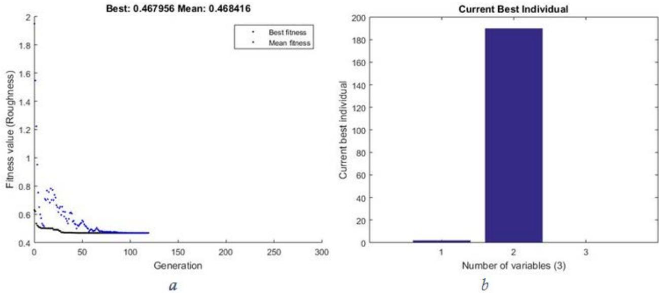
**Figure 6.** Optimal value selection of (a) surface roughness and (b) cutting speed using genetic algorithm
