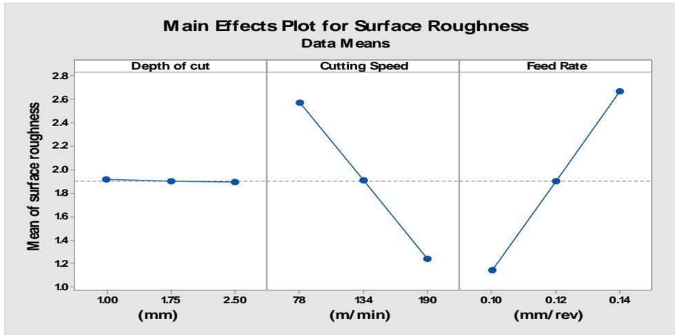
**Figure 2.** Main effects plot for surface roughness
