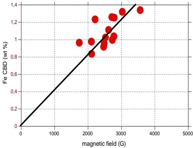
**Figure 4.** Evolution of iron after CBD treatment as a function of magnetic field for the fourteen Gounioubé's clays
