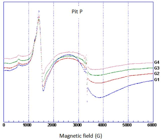
**Figure 2(a).** EPR Spectra of four kaolin samples from pit P of Gounioubé's deposit
