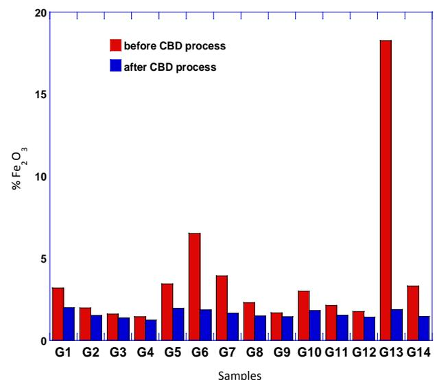
**Figure 3.** Comparison of content of ferric ion in kaolin samples of Gounioubé's deposit before and after CBD treatment
