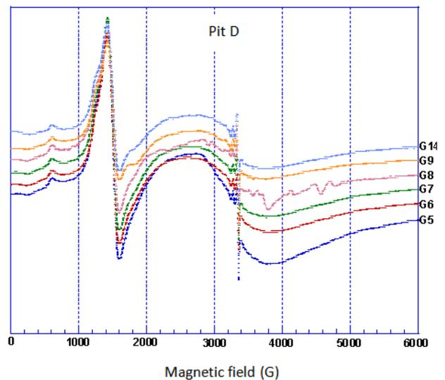
**Figure 2(b).** EPR Spectra of six kaolin samples from pit D of Gounioubé's deposit
