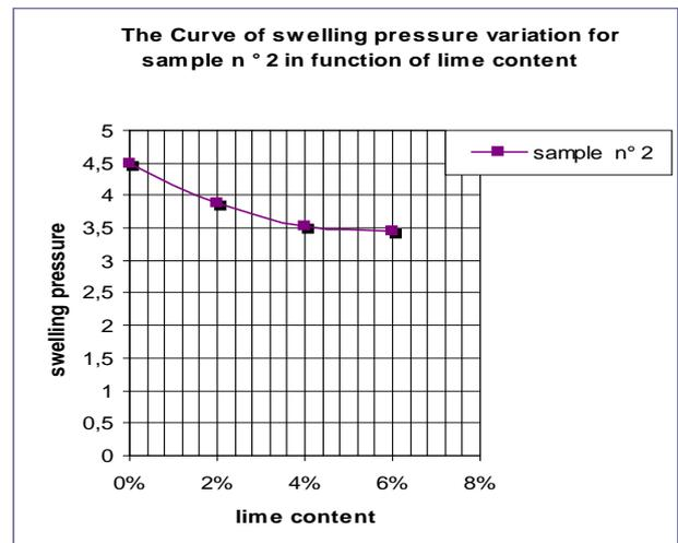
**Figure 8.** Curve of the variations of pressures of swelling of the sample 2 in function of proportionings lime
