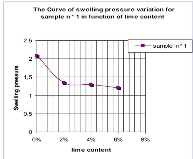
**Figure 7.** Curve of the variations of pressures of swelling of the sample 1 in function of proportionings lime
