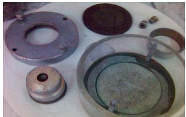
**Figure 1.** Components of the mould oedometric
