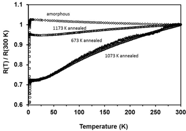
**Figure 3a.** The relative resistivity ( $\rho(T)/\rho(300K)$ ): amorphous ( $\diamond$ ), 673K annealed ( $\square$ ), 1073K annealed ( $\circ$ ), 1173K ( $\Delta$ )
