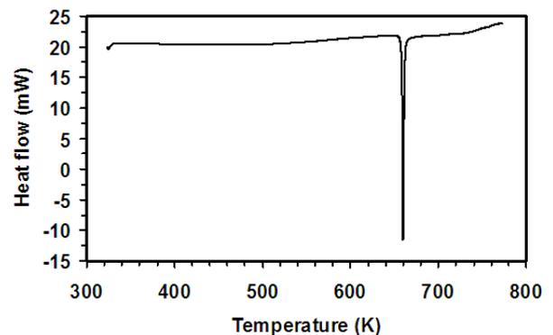
Figure 1. DSC trace of the Ni<sub>0.5</sub>Fe<sub>0.5</sub>Zr<sub>3</sub> metallic glass performed at a heating rate of 20K/min
