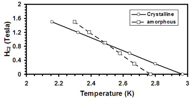
**Figure 4.**  $H_{c2}$  as a function of  $T_c$  for the amorphous (squares) and the 1073K annealed (circles) metallic glass at low temperatures
