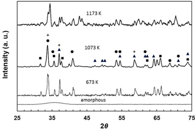
**Figure 2.** X-ray diffraction (XRD) profiles for different samples of Ni<sub>0.5</sub>Fe<sub>0.5</sub>Zr<sub>3</sub> metallic glass annealed over the temperature range 763 to 1173K for a period of two hours. (▲) fcc FeZr<sub>2</sub> and NiZr<sub>2</sub>, (■) bct FeZr<sub>2</sub>, (●) bct NiZr<sub>2</sub>, (+) Zr
