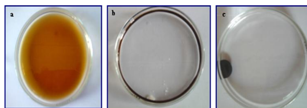
Figure 6. Represents the shape of petroleum film at water surface before addition of reagent (a); petroleum-dispersing shape after addition of reagent (b); petroleum-collection shape after addition of reagent (c)
