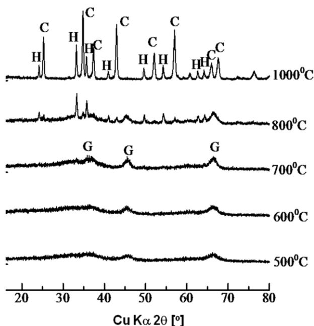
**Figure 3.** The XRD patterns of the 20 mol%  $\text{Fe}_2\text{O}_3$  CP samples heated at different calcination temperatures. Key: C =  $\alpha\text{-Al}_2\text{O}_3$ , G =  $\gamma\text{-Al}_2\text{O}_3$ , H =  $\alpha\text{-Fe}_2\text{O}_3$
