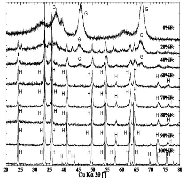
Figure 2(d). The XRD pattern of the samples heated at 800 °C for different Fe/(Fe+Al) ratio. Key: G =  $\gamma\text{-Al}_2\text{O}_3$ , H =  $\alpha\text{-Fe}_2\text{O}_3$
