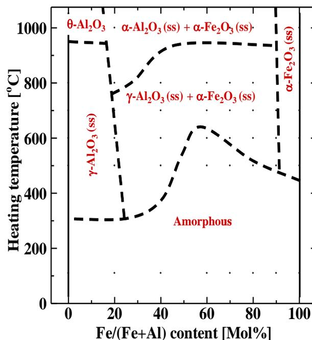
**Figure 4.** A field map of the phases formed in the samples as functions of composition and calcined temperature
