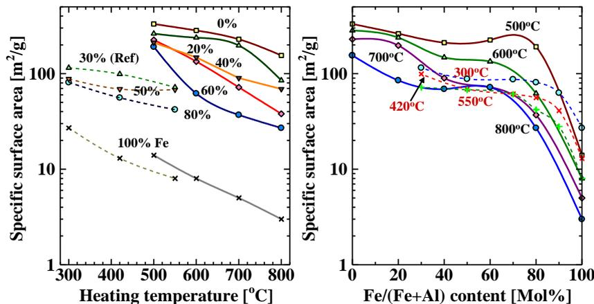
Figure 7. Changes in the  $S_{\text{BET}}$  values of the samples of various compositions as a function of heating temperature and  $\text{Fe}_2\text{O}_3$  content, together with the values reported by Li et al [11]
