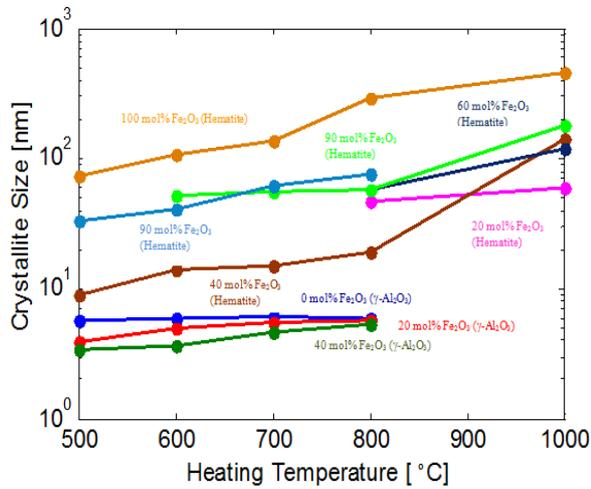
Figure 5. Crystallite size vs. temperature as a function of Fe/(Fe+Al)
