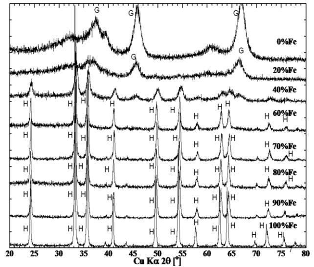
Figure 2(c). The XRD pattern of the samples heated at 700 °C for different Fe/(Fe+Al) ratio. Key: G =  $\gamma\text{-Al}_2\text{O}_3$ , H =  $\alpha\text{-Fe}_2\text{O}_3$
