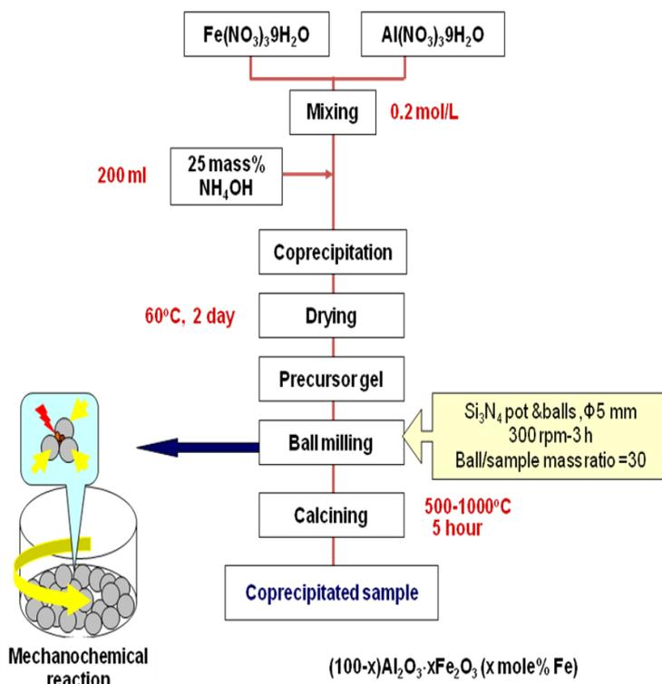
Figure 1. Flowchart for the preparation of  $\text{Al}_2\text{O}_3\text{-Fe}_2\text{O}_3$  compounds by coprecipitation method
