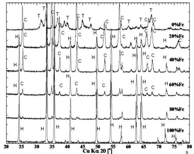
Figure 2(e). The XRD pattern of the samples heated at 1000 °C for different Fe/(Fe+Al) ratio. Key: C =  $\alpha\text{-Al}_2\text{O}_3$ , H =  $\alpha\text{-Fe}_2\text{O}_3$ , T =  $\theta\text{-Al}_2\text{O}_3$
