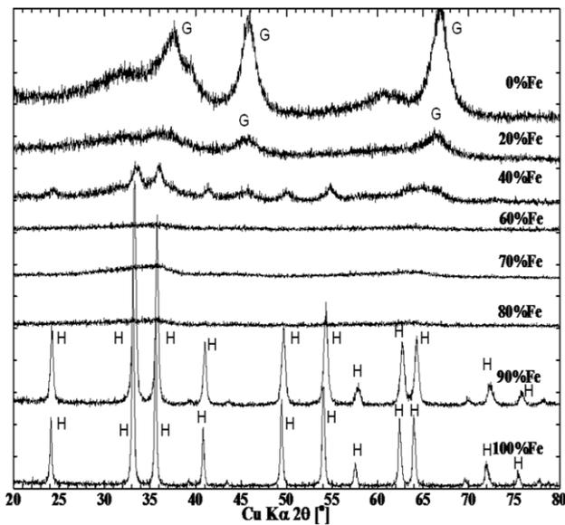
Figure 2(a). The XRD pattern of the samples heated at 500 °C for different Fe/(Fe+Al) ratio. Key: G =  $\gamma\text{-Al}_2\text{O}_3$ , H =  $\alpha\text{-Fe}_2\text{O}_3$
