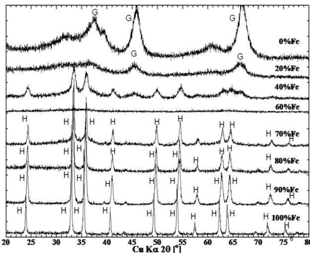
Figure 2(b). The XRD pattern of the samples heated at 600 °C for different Fe/(Fe+Al) ratio. Key: G =  $\gamma\text{-Al}_2\text{O}_3$ , H =  $\alpha\text{-Fe}_2\text{O}_3$
