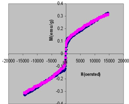
Figure 6. Magnetization curves of 80 mol%  $\text{Fe}_2\text{O}_3$  CP sample calcined at 800 °C [blue line] and that at 1000 °C [pink line]
