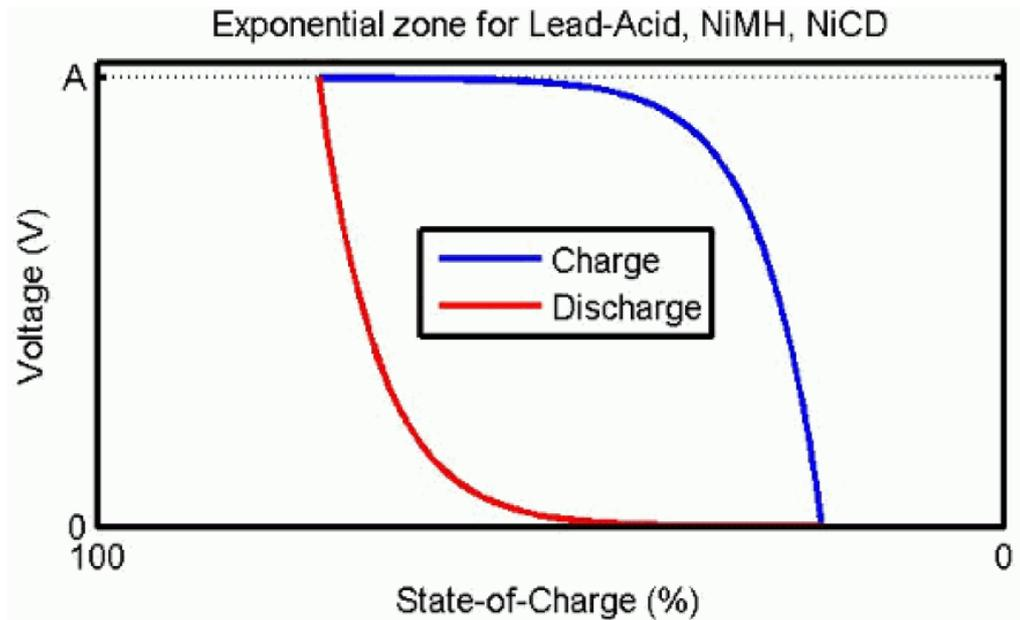
Figure 6. Exponential zone for lead –acid, NI-MH and NiCD
