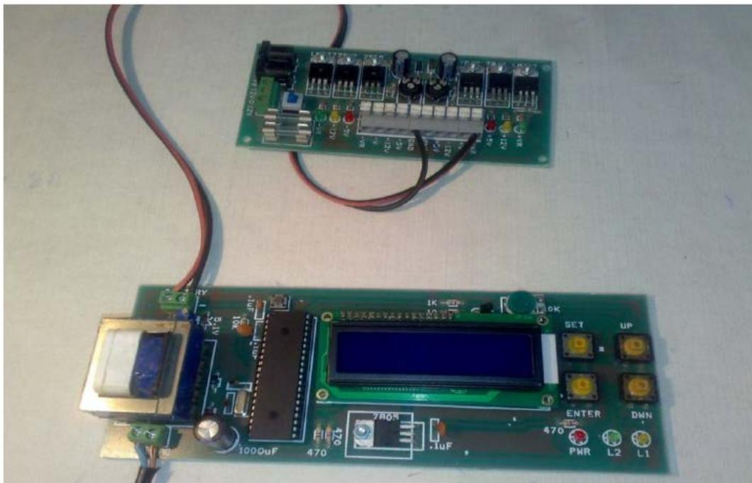
Figure 10. Measurement device and Voltage simulator
