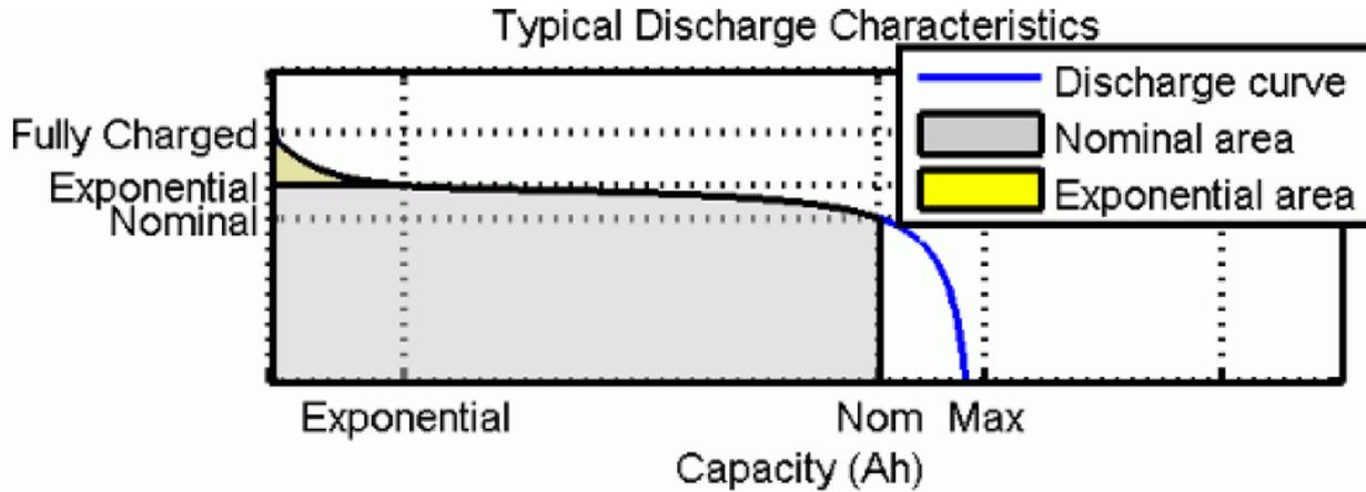
Figure 4. Typical discharge characteristics
