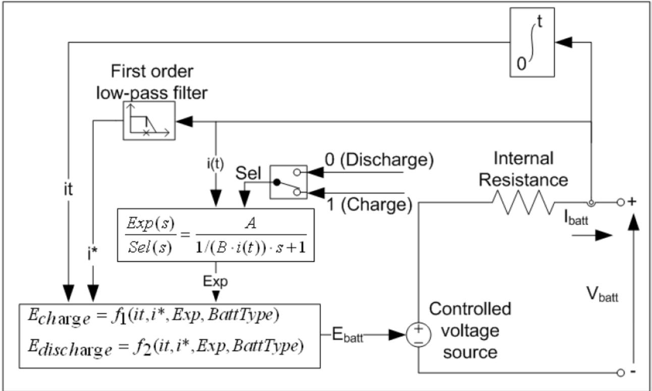
Figure 3. The equivalent circuit of the battery
