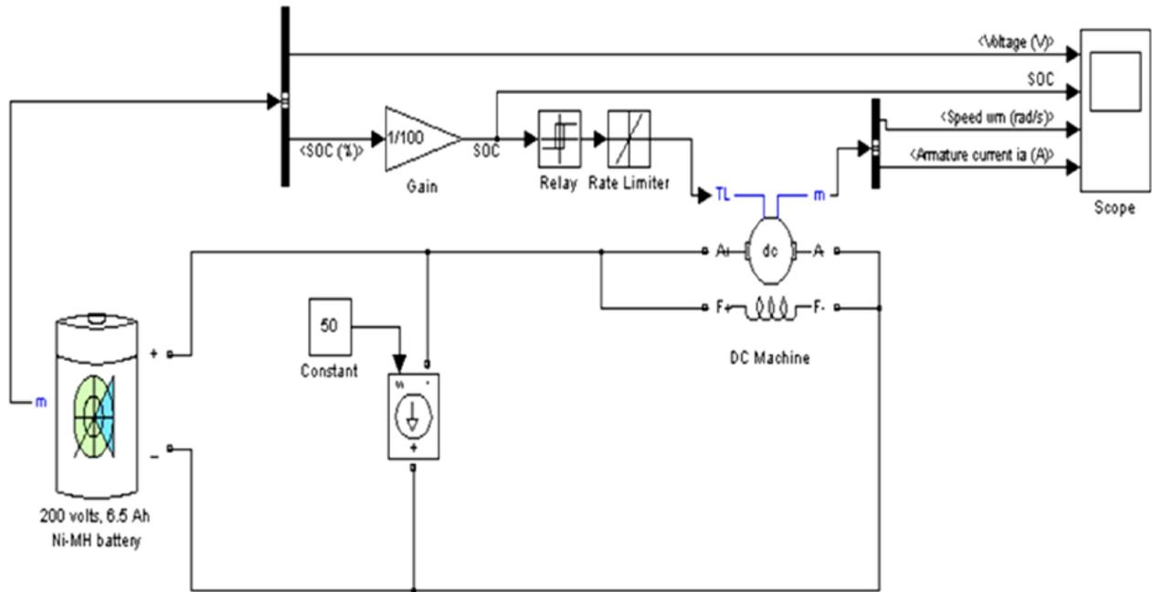
Figure 7. Simulation Model in SIMULINK for Vehicle nickel hydrogen battery (NiMH)
