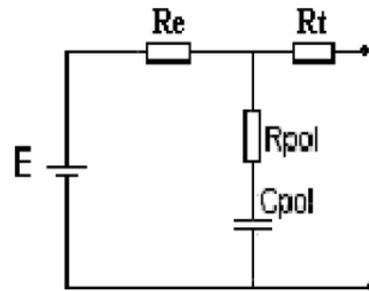
Figure 1. Battery model
