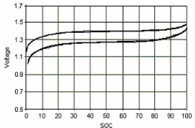
Figure 2. Charge and discharge curves for NiMH
