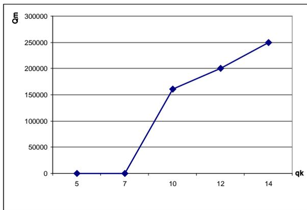
**Figure 4.** Changing of intensity of particles entrainment depending on the soda carbonate content in soil
