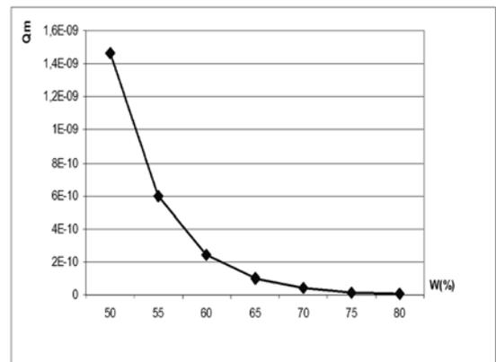
Figure 1. Changing of intensity of particles entrainment  $\theta$  depending on levels of soil moisture  $w$
