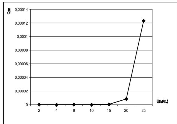
Figure 2. Changing of intensity of particles entrainment  $\theta$  depending on the flow speed  $u$
