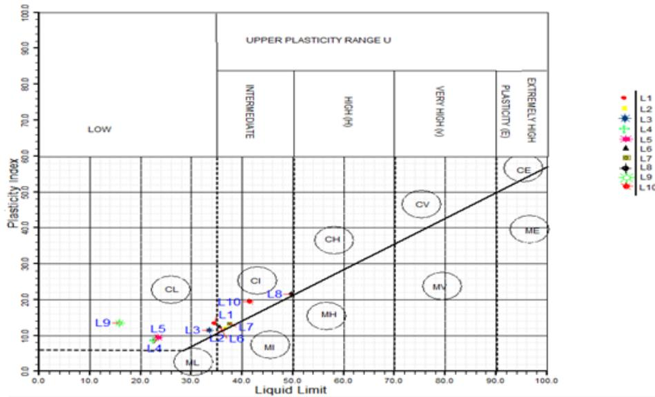
**Figure 4. Plasticity chart of the Atterberg limits result**
