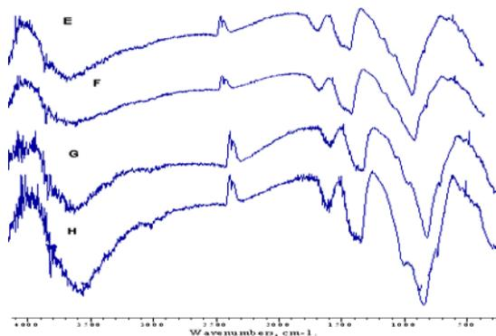
**Figure 11.** The FTIR spectra of LPC pastes cured up to 90 days (a), premixed with 1 % PWL (b), 2 wt. % PWL (c) and 3 wt. % PWL (d)
