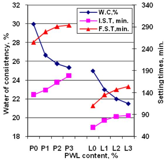
Figure 2. Water of consistency and setting times of the OPC and PLC cement pastes premixed with 0, 1, 2 and 3 wt. % PWL waste
