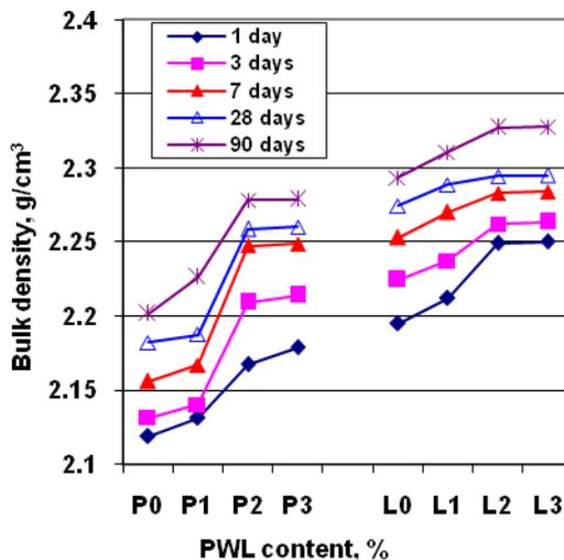
Figure 3. Bulk density of the OPC and PLC cement pastes premixed with 0, 1, 2 and 3 wt. % PWL waste cured up to 90 days
