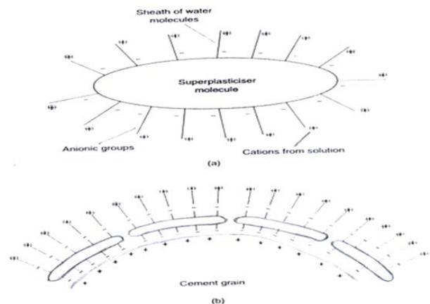
Figure 9. (a) Representation of an admixture molecule and (b) Mode of adsorption of admixture on cement grain
