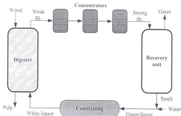
Figure 1. A schematic description of the pulping process
