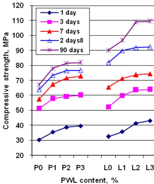
Figure 6. Compressive strength of OPC and PLC pastes premixed with 0, 1, 2 and 3 wt. % PWL waste cured up to 90 days
