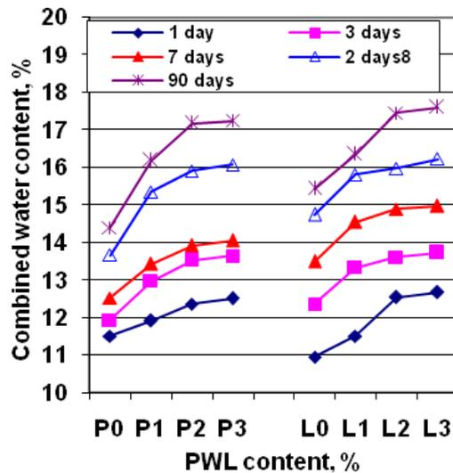
Figure 5. Combined water content of OPC and PLC pastes premixed with 0, 1, 2 and 3 % PWL waste cured up to 90 days
