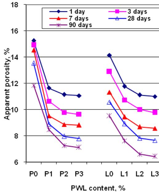
Figure 4. Apparent porosity of the OPC and PLC pastes premixed with 0, 1, 2 and 3 wt. % PWL waste cured up to 90 days
