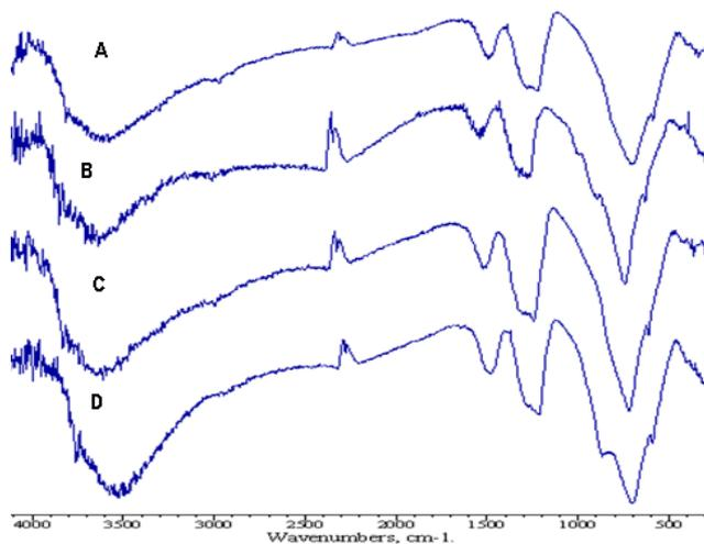
**Figure 10.** The FTIR spectra of OPC pastes cured up to 90 days (a), premixed with 1 wt. % PWL (b), 2 wt. % PWL (c) and 3 wt. % PWL (d)
