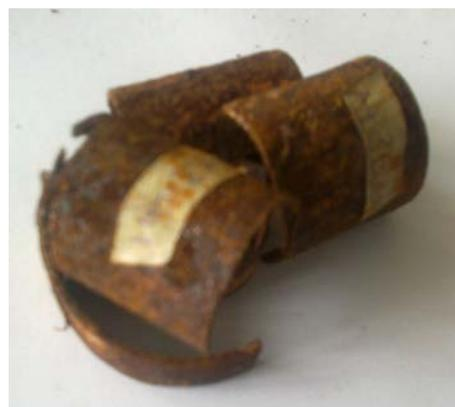
Figure 2. Corroded pieces of galvanized steel cut and exposed to sea water environment
