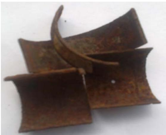
Figure 2. Corroded pieces of Al-Mn alloy cut and exposed to sea water environment
