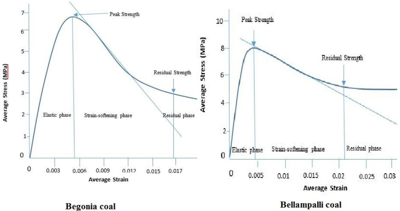
Figure 5. Average strain and average stress curve for Begonia coal and Bellampalli coal
