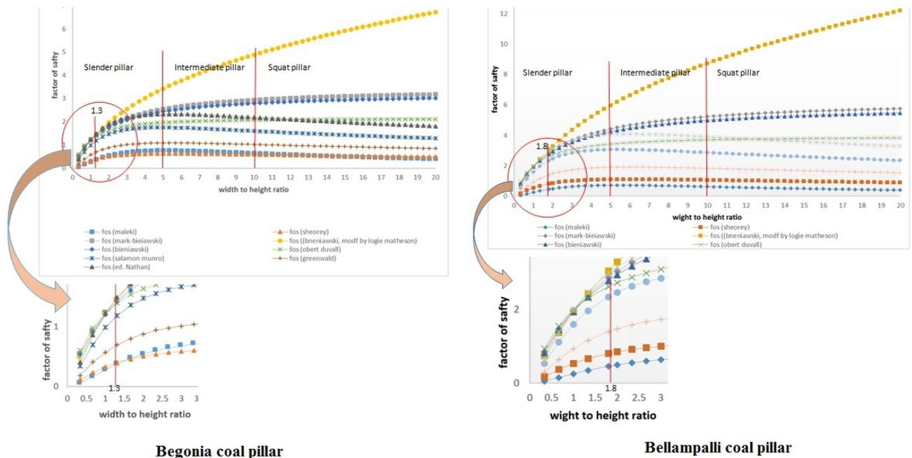
Figure 6. Variation of Begonia coal pillar and Bellampalli coal pillar FOS with w/h ratio
