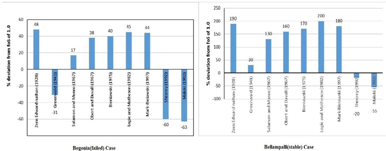
**Figure 3.** percentage deviation from FOS of 1.0 for Begonia (failed case) and Bellampalli (stable case) by different empirical relation
