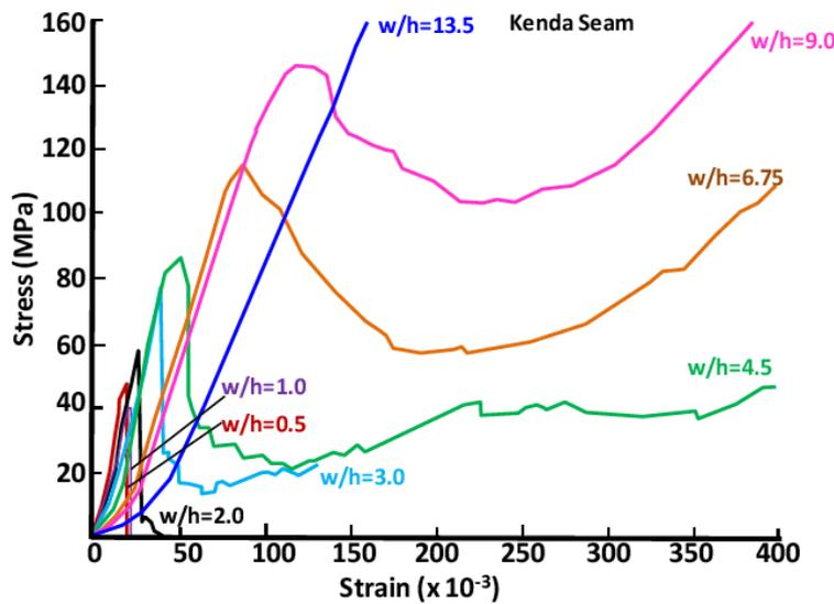
Figure 1. Influence of w/h ratio on the post-failure stress-strain behavior of coal (Das, 1986)
