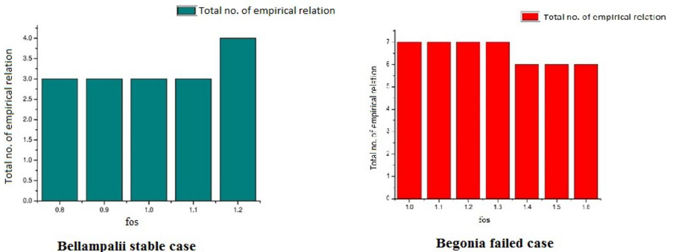
**Figure 4.** Number of empirical relation predicting stable cases and failed cases at different critical FOS
