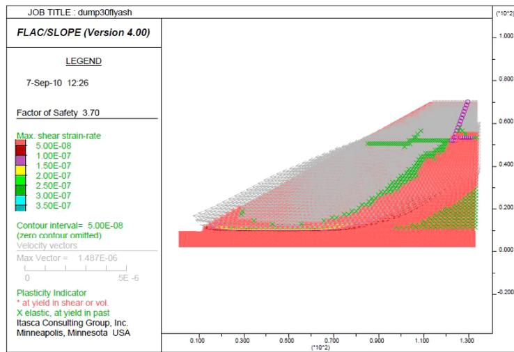
Figure 3. Simulated model for dump slope with H = 60m and slope angle = 30°
