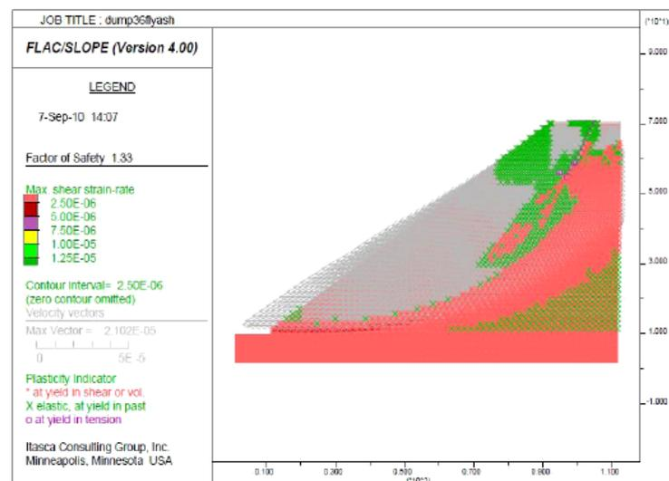
Figure 6. Simulated model for dump slope with H = 60m and slope angle = 36°
