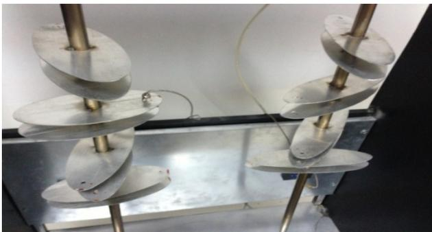
**Figure 1.** Elliptical fin shape at different axis used in the experimental work for natural convection
