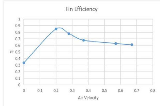
**Figure 6.** Elliptical fin efficiency ( $\eta$ ) with air fan velocities
