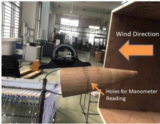
Figure 3. Position of the projectiles against the wind and measurement of the pressure at the tapping points of the projectile. (Fluid Mechanics Lab of MIST)
