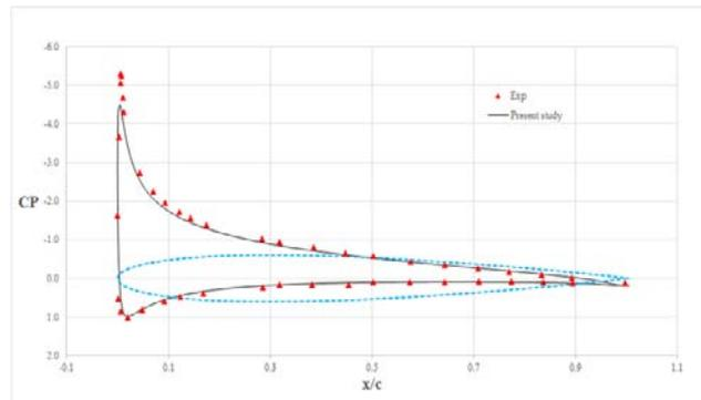
Figure 5. Pressure coefficient distribution for NACA0012 in angle of attack  $\alpha_0=10^\circ$
