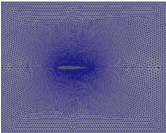
Figure 10. Computational domain for FVS with 18706 cells.
