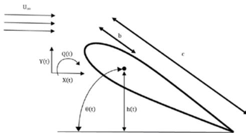
Figure 2. Geometry of the foil and lift, drag and moment about its pivot point
