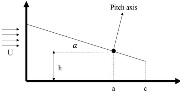
Figure 7. Oscillating pitch and heave motion of a flat plate.
