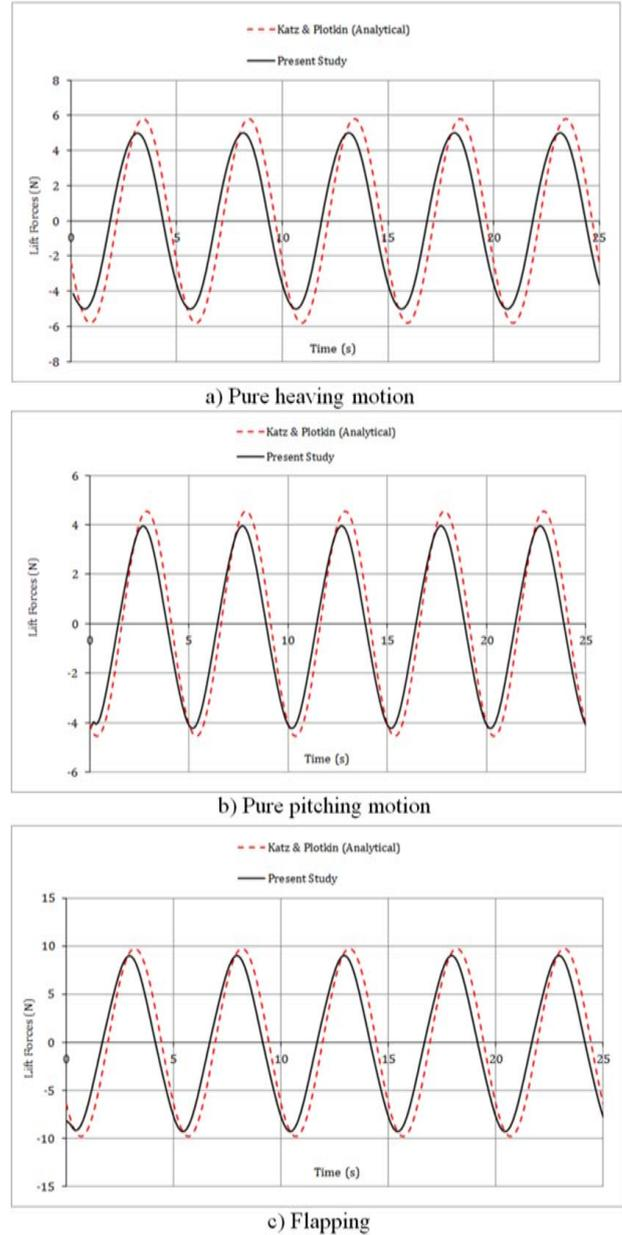
Figure 9. Lift forces for the oscillating foil
