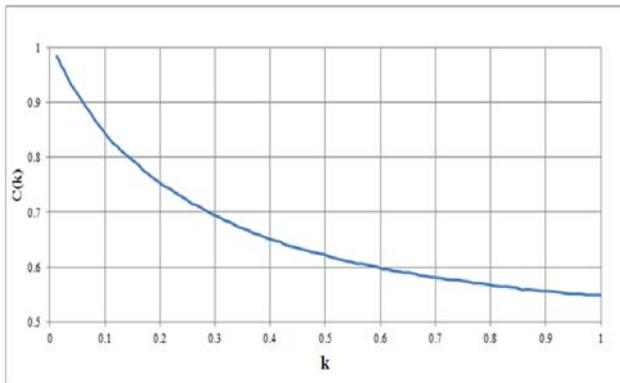
Figure 8. Lift deficiency versus reduced frequency.
