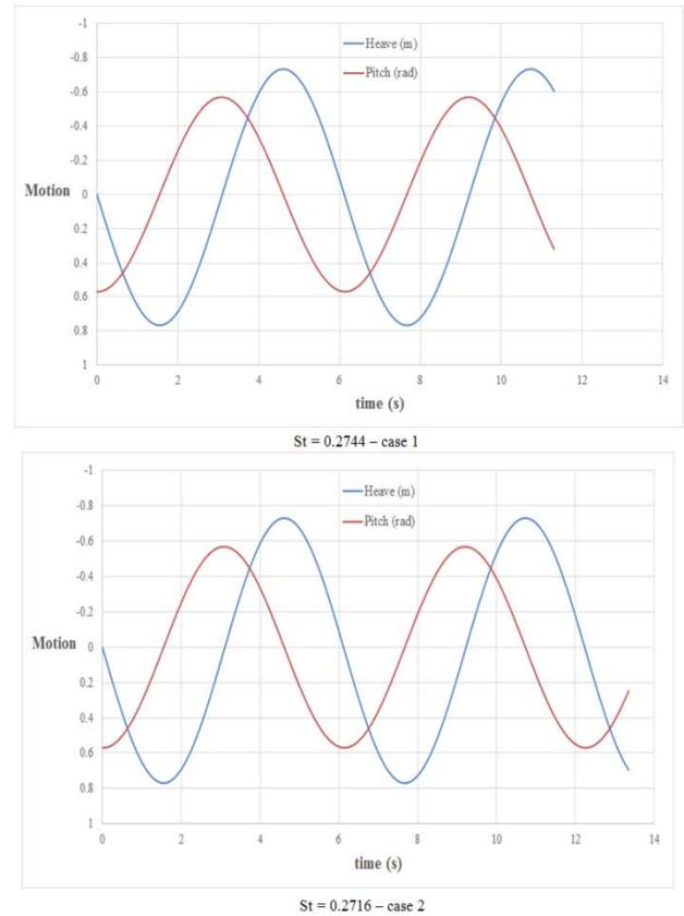
Figure 11. Heave and pitch motions of air foil
