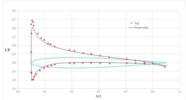
Figure 4. Pressure coefficient distribution for NACA0012 in angle of attack  $\alpha_0=6^\circ$
