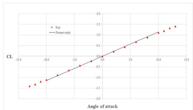
Figure 6. Lift coefficient for NACA0012 in angle of attack  $\alpha_0=10^\circ$
