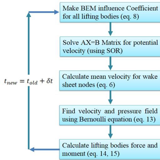
Figure 1. Applied algorithm for BEM solver
