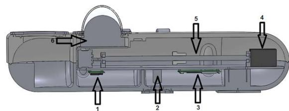
Figure 7. Locating internal components: (1) Sensors, (2) Bottom camera, (3) Mini-PC, (4) Batteries (5) Mass Shifter, (6) Main Camera
