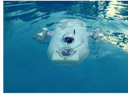
Figure 16 The final prototype of AUV in operation on water. At this time, the user is sending it the commands to begin its mission
