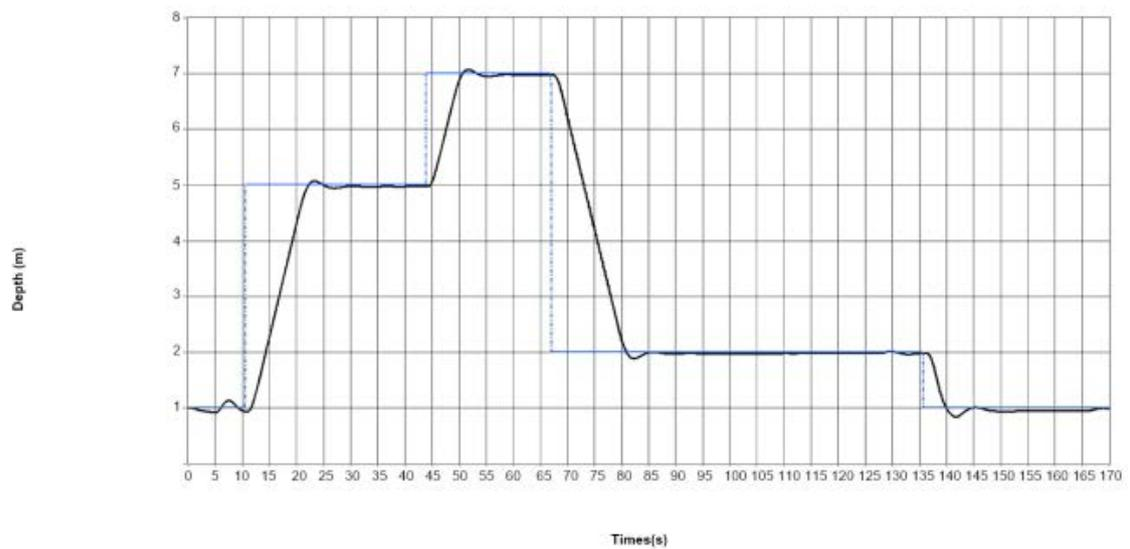
Figure 26. AUV response (Black) to depth command (Blue)
