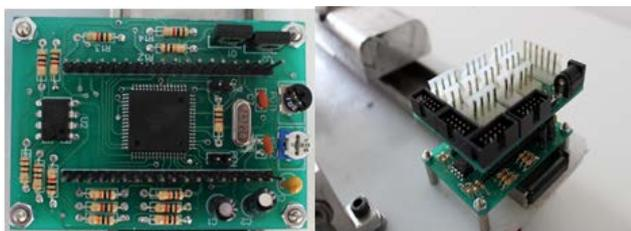
Figure 10. Sensor board (top board of dimensions 67.4\*48.4 mm<sup>2</sup> and bottom board of dimensions 69.8\*49.8 mm<sup>2</sup>)
