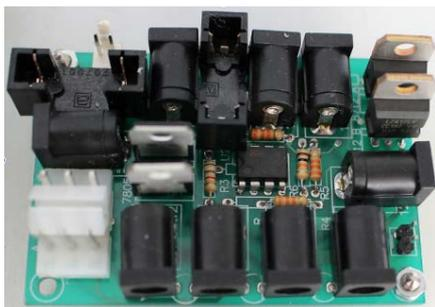
Figure 12. Power Distribution Board
