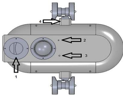
Figure 3. Access valve (1), Antenna holes (2), Pressure sensor (3), and Dolly block of servo motor (4)
