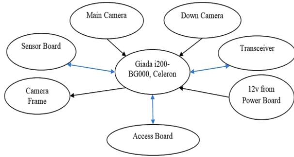
Figure 8. Block diagram of main processor
