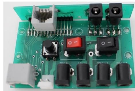
Figure 13. Access Valve Board with dimensions 52.4\*87.4 mm<sup>2</sup>
