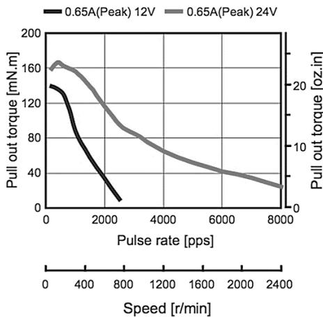
**Figure 15.** Dynamic torque curves of the Moons hybrid stepper motor 16HS Series 1.8°/12 V DC [1,16]
