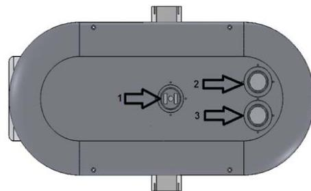
Figure 6. The Bottom openings: (1) Bottom camera, (2) and (3) Sensors
