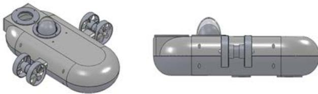
Figure 2. Different views of the designed AUV
