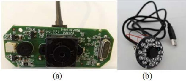
Figure 11. (a): The Main Camera Board and (b): The Down Camera
