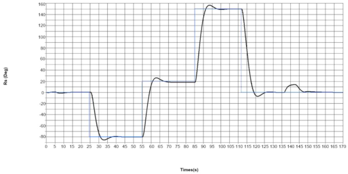
Figure 27. AUV response (Black) to direction angle command (Blue).
