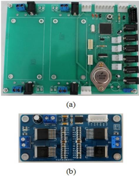
**Figure 14.** Engine driver board with dimensions 157.5\*12 mm<sup>2</sup>, (b) BTN7971B driver module
