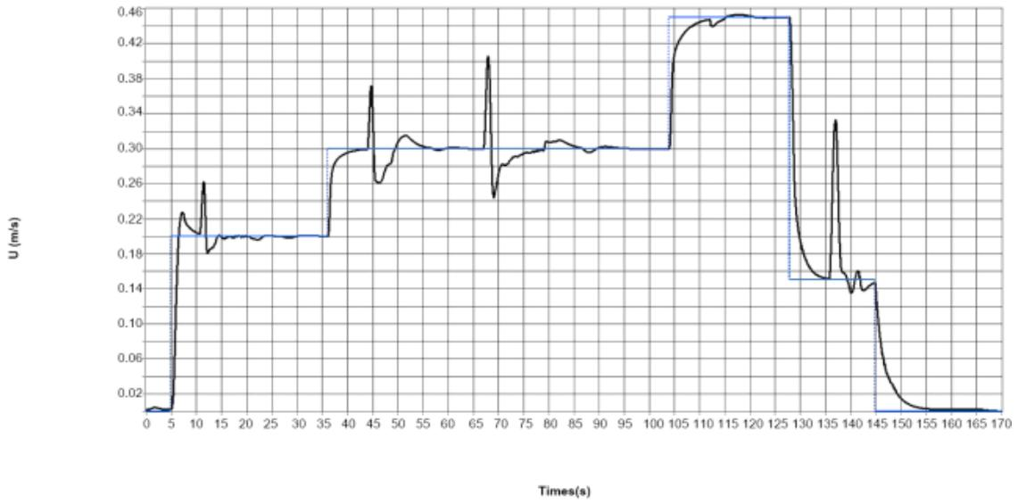
Figure 21. AUV response (Black) to speed command (Blue)
