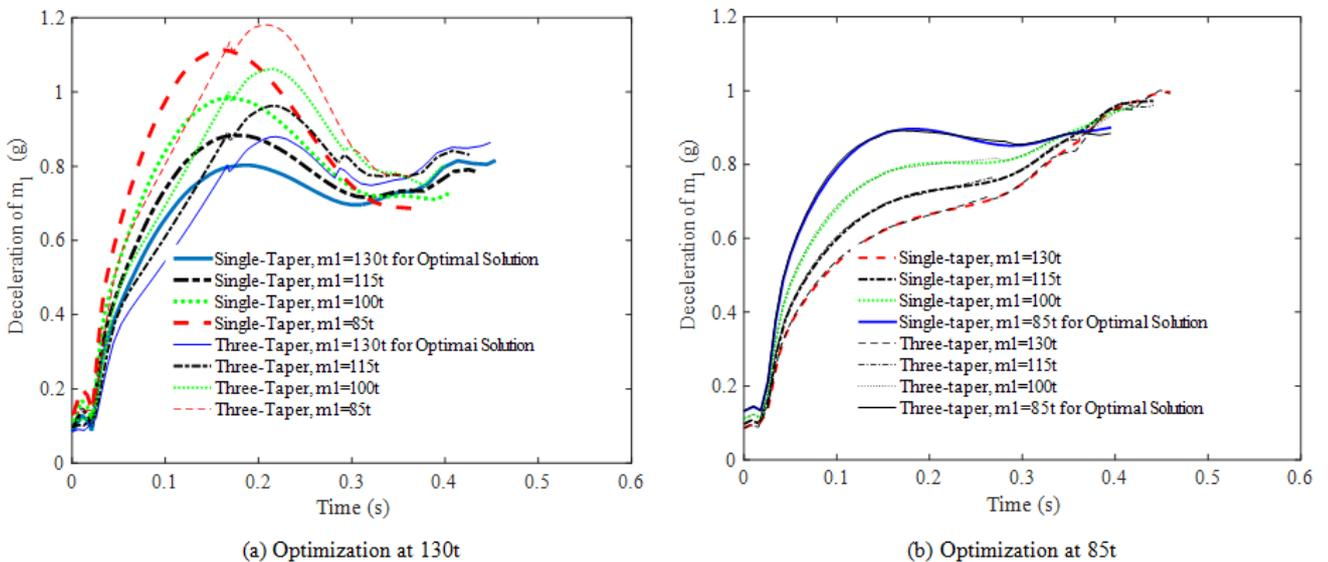
Figure 9. Comparison of single-taper and three-taper for optimization at 130t and 85t
