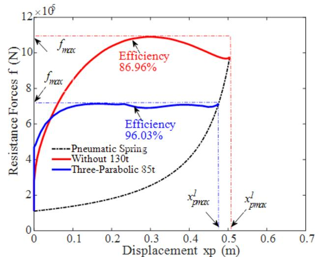
Figure 12. Efficiency for shock absorbers
