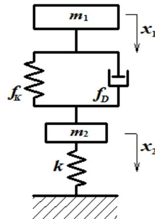
Figure 4. Model of an aircraft landing gear
