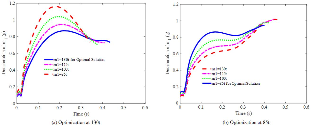
Figure 7. Simulation of accelerations for shock absorber without metering pin
