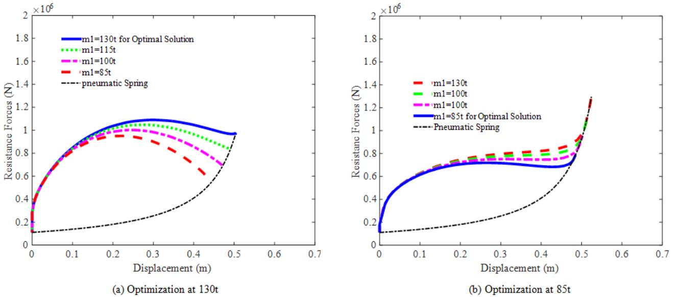
Figure 8. Simulation of resistance forces for shock absorber without metering pin
