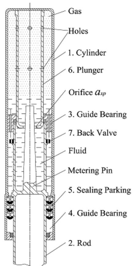
Figure 2. Schematic diagrams of passive shock absorber with metering pin
