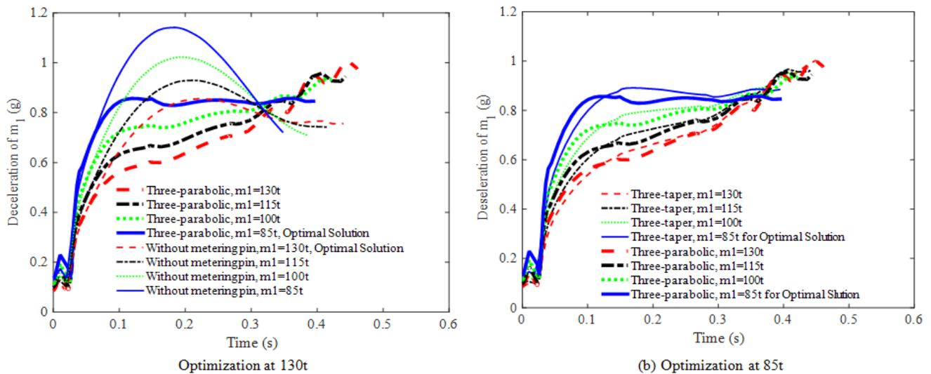
Figure 11. Comparison of three-parabolic and without metering pin for optimization at 130t and 85t
