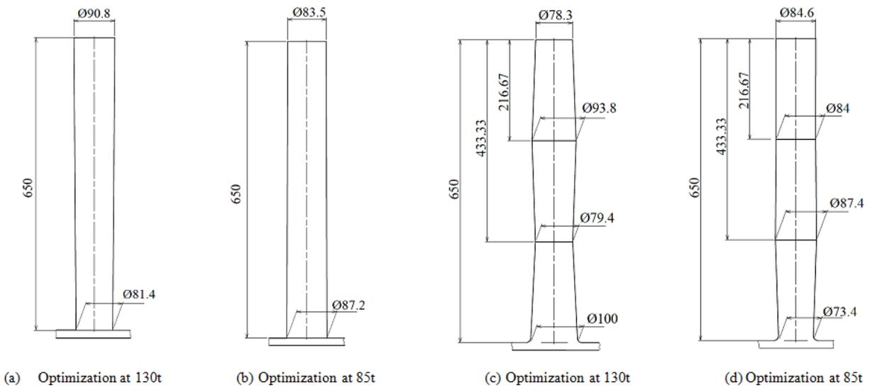
Figure 5. Diagrams of metering pins with single and three-tapered profile using optimal solutions
