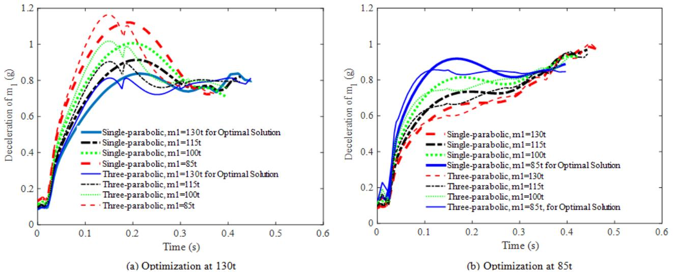
Figure 10. Comparison of single-parabolic and three-parabolic for optimization at 130t and 85t
