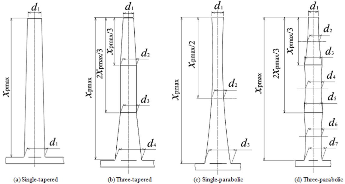
Figure 3. Schematic diagrams of the metering pin constructions
