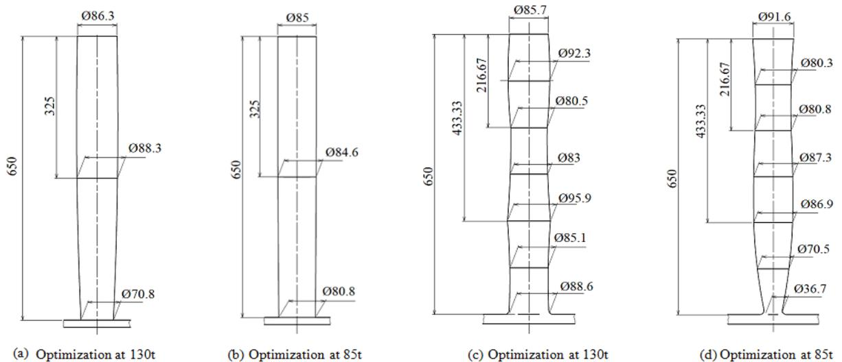
Figure 6. Diagrams of metering pins with single and three parabolic profiles using optimal solutions
