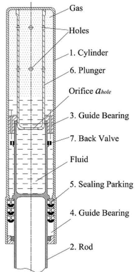
Figure 1. Schematic diagrams of passive shock absorber without metering pin
