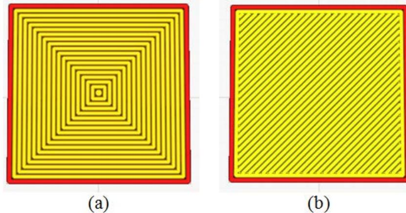
Figure 4. Concentric pattern with 100% infill (a) without top/bottom thickness (b) with a top/bottom thickness
