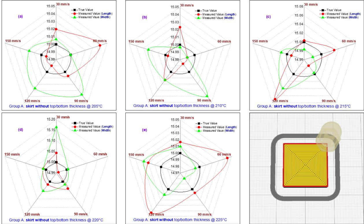
Figure 6. Length versus width variation including true and measured values of group A (skirt without top/bottom thickness)
