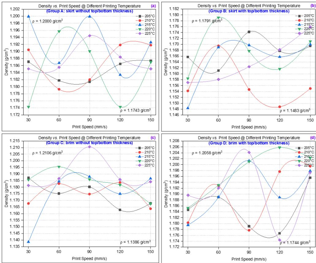
Figure 18. Density versus print speed @ different printing temperature (a) skirt without top/bottom thickness, (b) skirt with top/bottom thickness, (c) brim without top/bottom thickness and (d) brim with a top/bottom thickness
