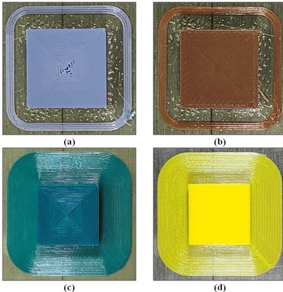
**Figure 5.** Fabricated model of PLA Plus (a) skirt without top/bottom thickness, (b) skirt with top/bottom thickness, (c) brim without top/bottom thickness and (d) brim with a top/bottom thickness
