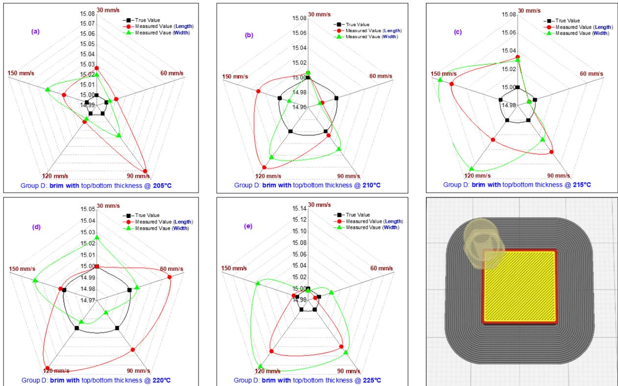
Figure 9. Length versus width variation including true and measured values of group D (brim with a top/bottom thickness)
