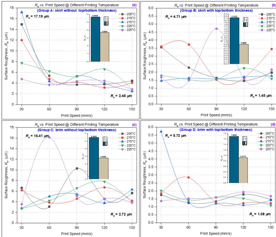
**Figure 14.** Surface roughness versus print speed @ different printing temperature (a) skirt without top/bottom thickness, (b) skirt with top/bottom thickness, (c) brim without top/bottom thickness and (d) brim with a top/bottom thickness
