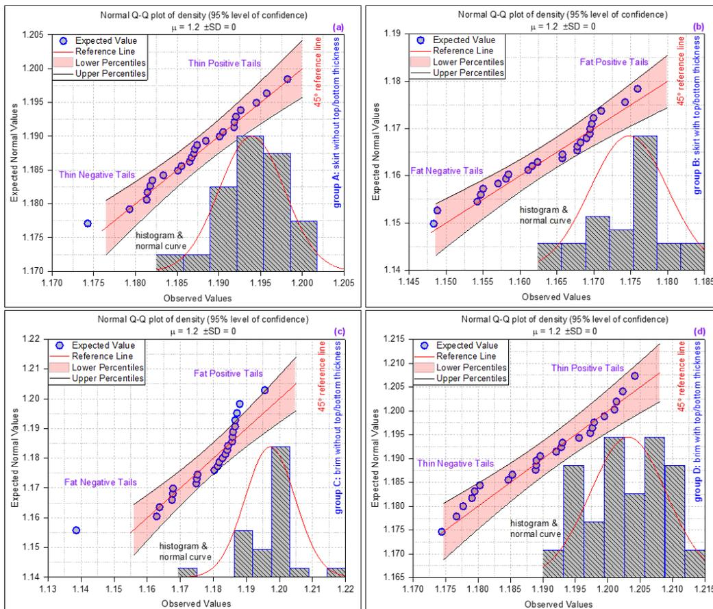
Figure 19. Normal Q-Q (quantile-quantile) plot of density between experimental data and expected data (a) skirt without top/bottom thickness, (b) skirt with top/bottom thickness, (c) brim without top/bottom thickness and (d) brim with a top/bottom thickness
