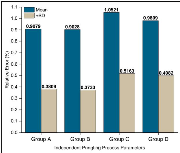
**Figure 11.** Relative error of (group A: skirt without top/bottom thickness), (group B: skirt with top/bottom thickness), (group C: brim without top/bottom thickness and (group D: brim with a top/bottom thickness)
