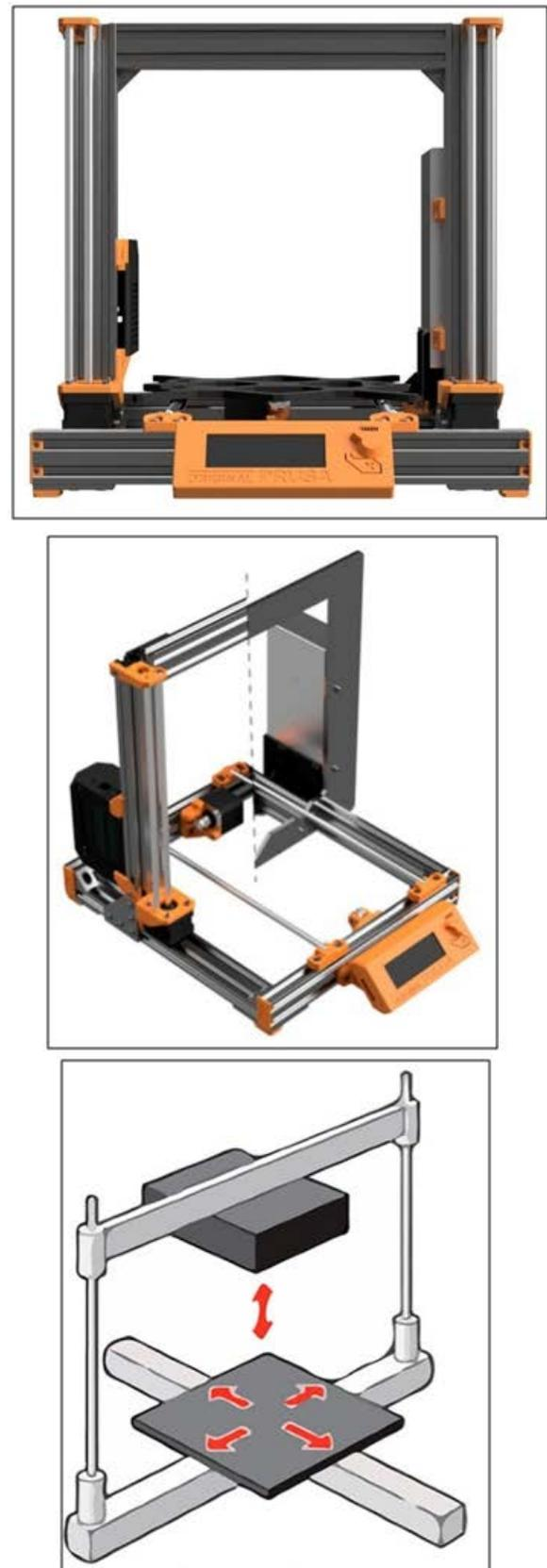
Figure 1. Cartesian configuration (square stage), adapted from [31]
