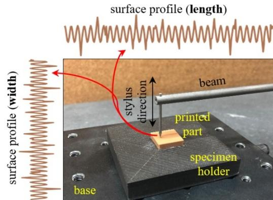
**Figure 12.** Image of Taly-surf<sup>®</sup> with conisphere tip  $r = 2 \mu\text{m}$  (from Taylor Hobson) and specimen holder with a located specimen correctly positioned within a precision machine
