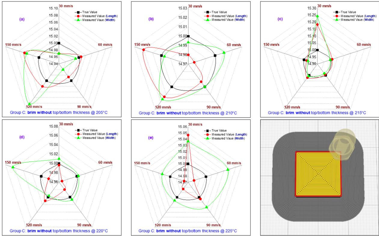
Figure 8. Length versus width variation including true and measured values of group C (brim without top/bottom thickness)
