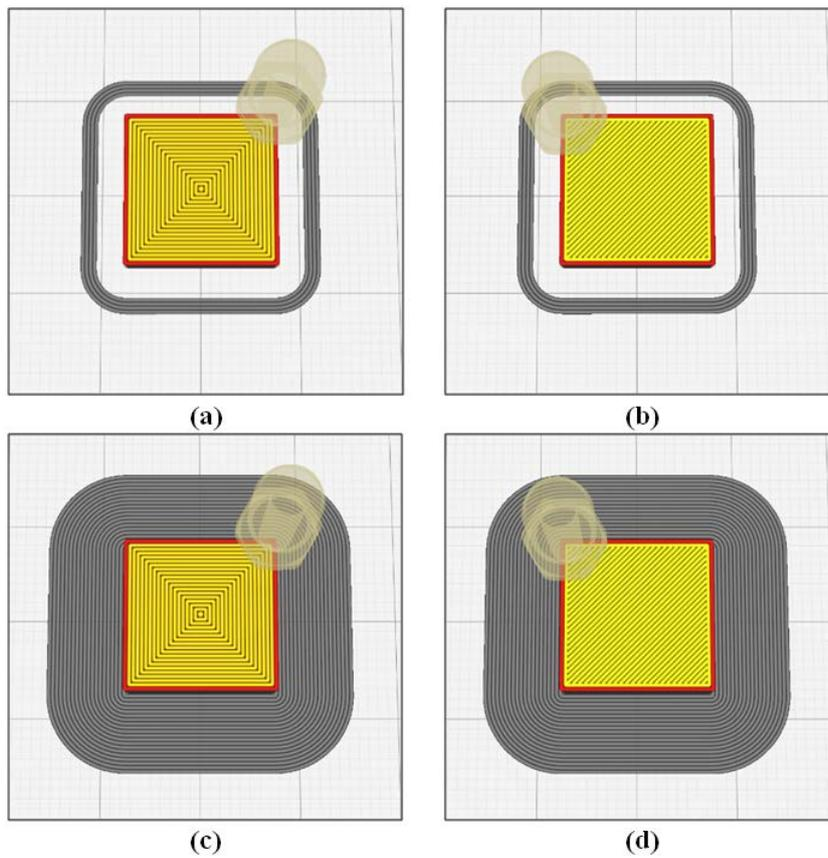
Figure 3. Cura software using 100% infill density of PLA Plus (a) skirt without top/bottom thickness, (b) skirt with top/bottom thickness, (c) brim without top/bottom thickness and (d) brim with a top/bottom thickness
