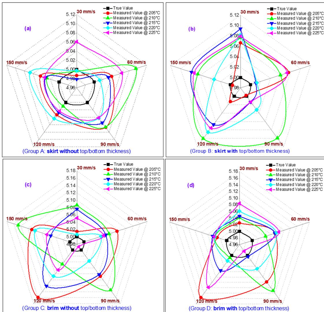
Figure 10. Height variation including true and measured values (a) skirt without top/bottom thickness, (b) skirt with top/bottom thickness, (c) brim without top/bottom thickness and (d) brim with a top/bottom thickness
