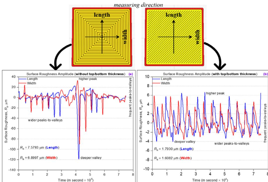
Figure 13. Surface roughness height profile of length and width (a) without top/bottom thickness and (b) with a top/bottom thickness
