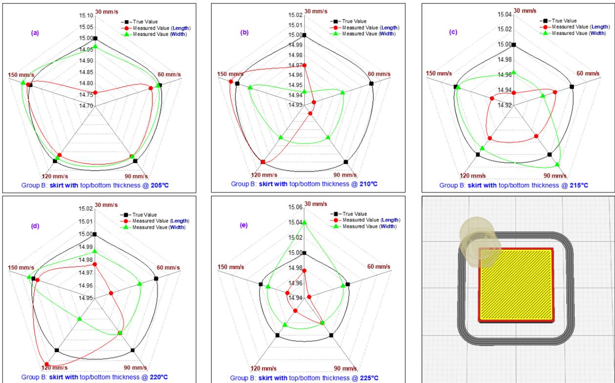
Figure 7. Length versus width variation including true and measured values of group B (skirt with top/bottom thickness)
