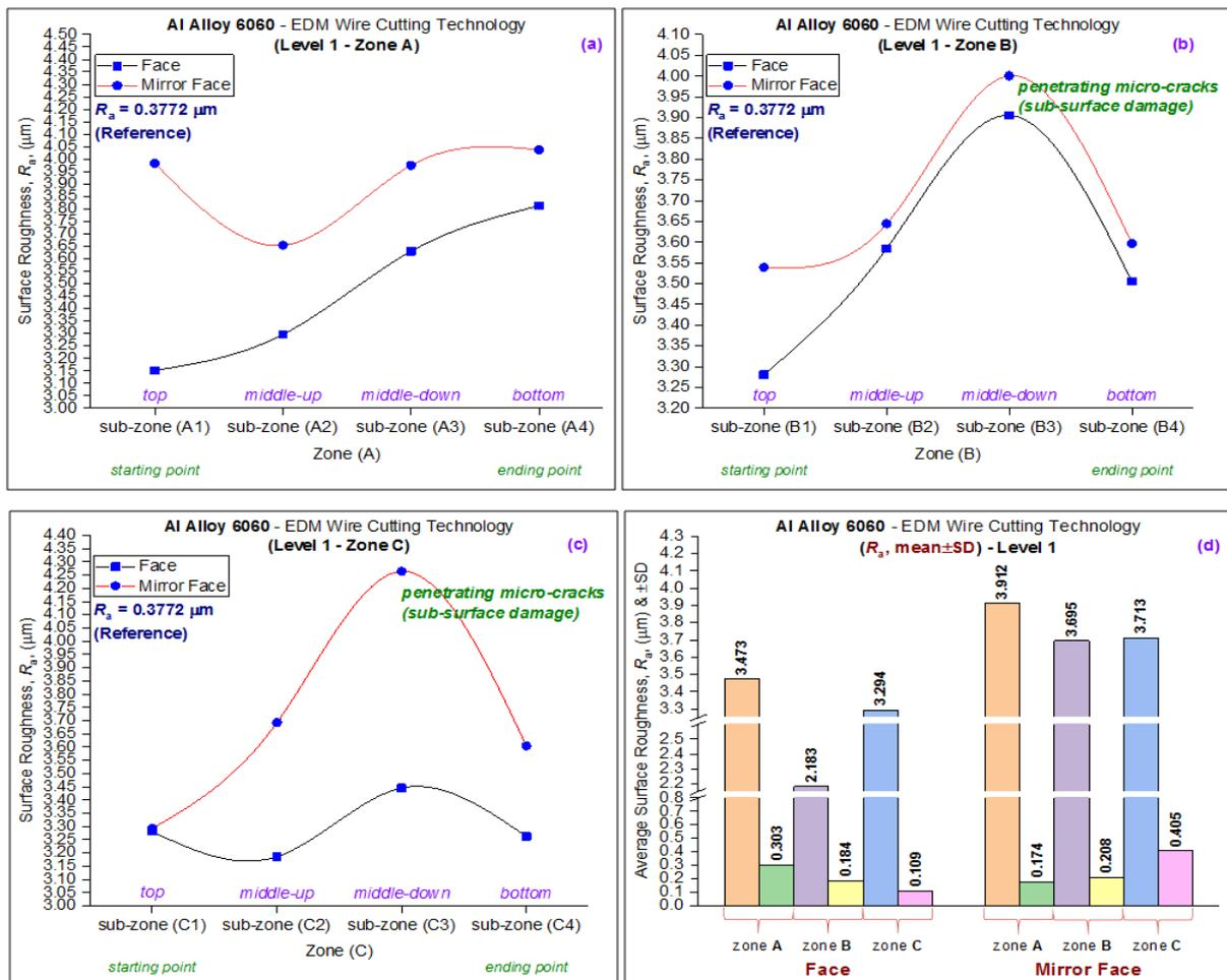
Figure 8. Surface roughness of aluminum alloy 6060 at level 1 parameters with different zones (a) zone A, (b) zone B, (c) zone C and (d) average surface roughness with a standard deviation
