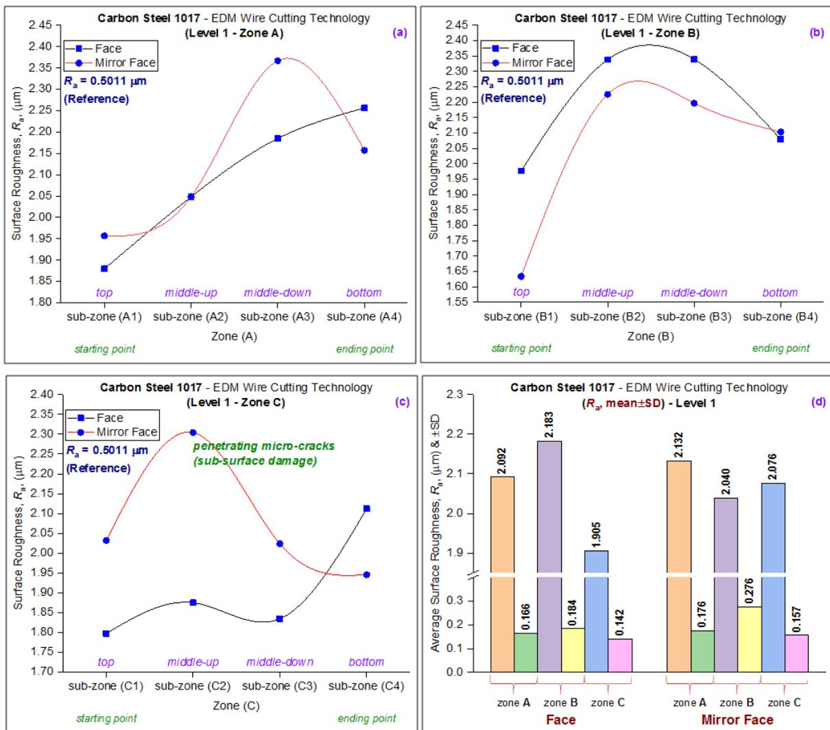
Figure 5. Surface roughness of carbon steel 1017 at level 1 parameters with different zones (a) zone A, (b) zone B, (c) zone C and (d) average surface roughness with a standard deviation
