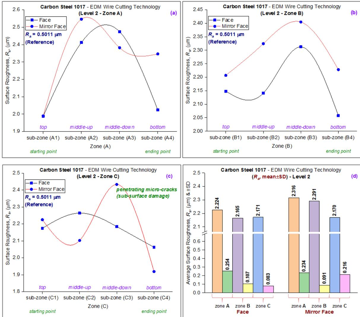
**Figure 6.** Surface roughness of carbon steel 1017 at level 2 parameters with different zones (a) zone A, (b) zone B, (c) zone C and (d) average surface roughness with a standard deviation
