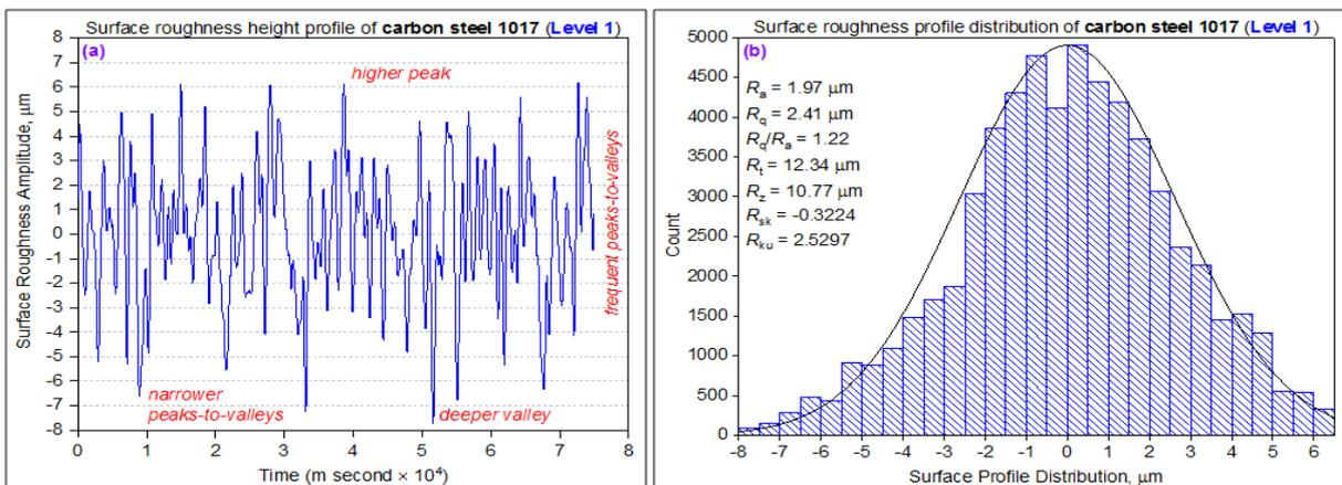
Figure 3. Surface roughness profile of carbon steel 1017 (a) height profile and (b) distribution profile
