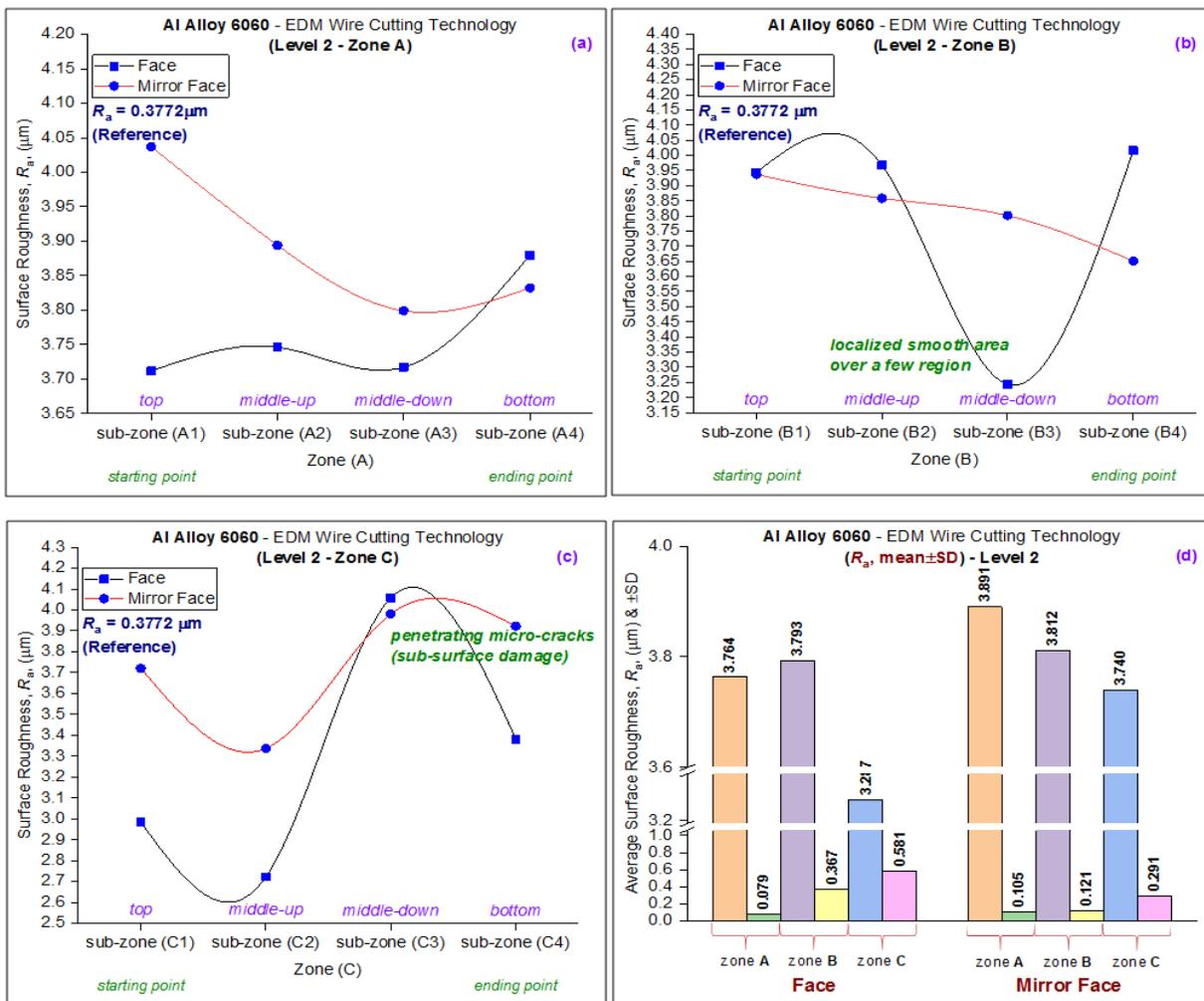
Figure 9. Surface roughness of aluminum alloy 6060 at level 2 parameters with different zones (a) zone A, (b) zone B, (c) zone C and (d) average surface roughness with a standard deviation
