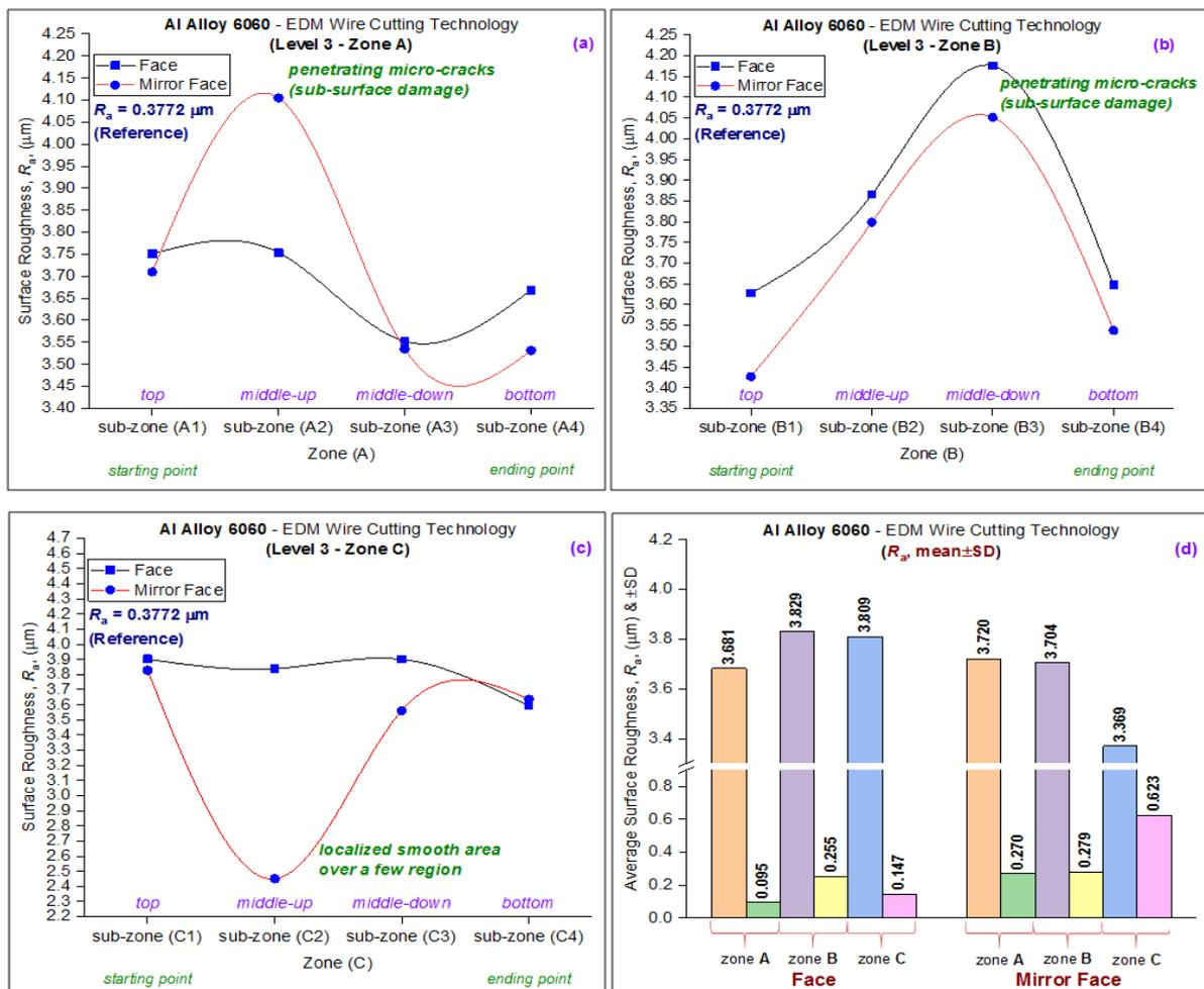
Figure 10. Surface roughness of aluminum alloy 6060 at level 3 parameters with different zones (a) zone A, (b) zone B, (c) zone C and (d) average surface roughness with a standard deviation
