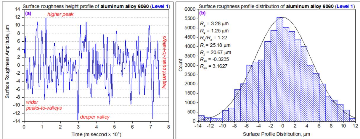
**Figure 4.** Surface roughness profile of aluminum alloy 6060 (a) height profile and (b) distribution profile
