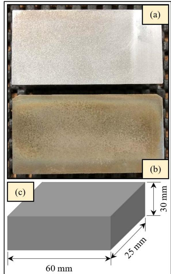
Figure 1. Photo of the (a) aluminum alloy 6060, (b) carbon steel 1017 and (c) 3D schematic object
