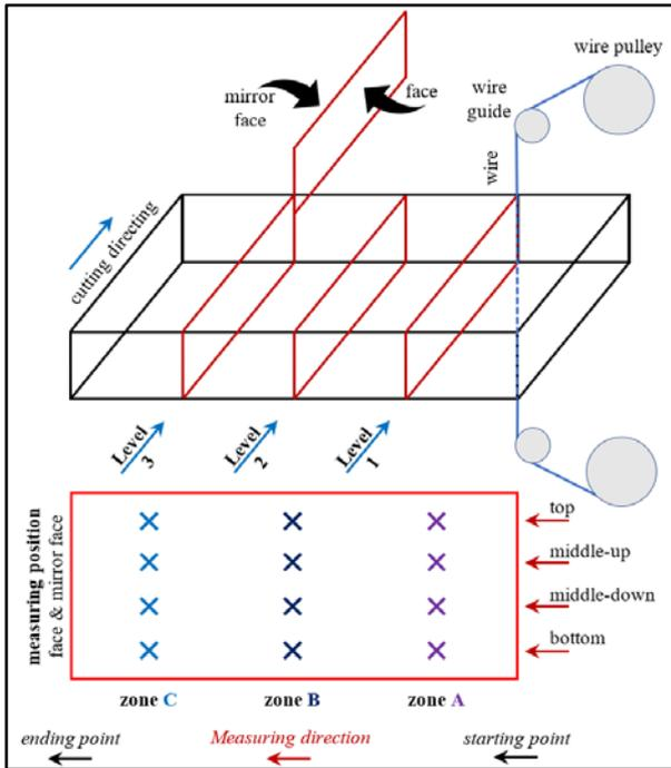
Figure 2. Schematic diagram of the sample design and measuring technique
