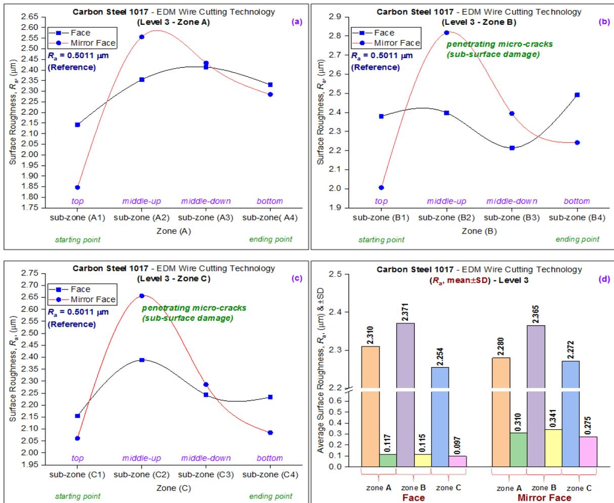
Figure 7. Surface roughness of carbon steel 1017 at level 3 parameters with different zones (a) zone A, (b) zone B, (c) zone C and (d) average surface roughness with a standard deviation
