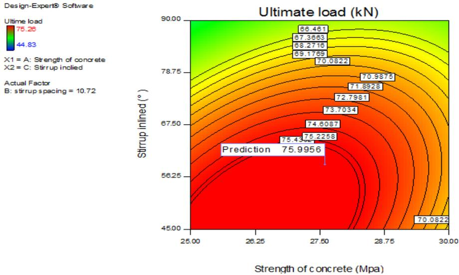
(b) Stirrup inclined=58.94°, strngth concrete =27.60 MPa
