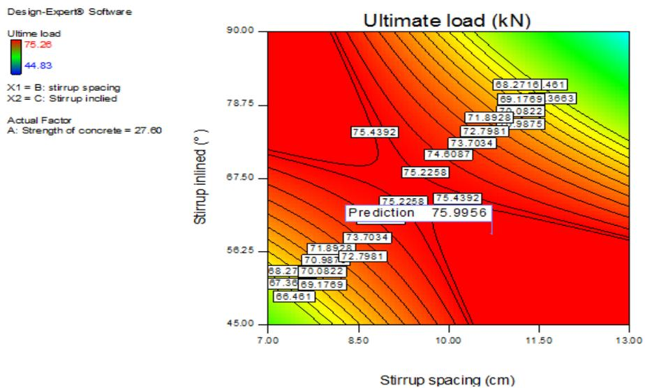
(c) Stirrup spacing = 10.71 cm, stirrup inclined=58.94°
