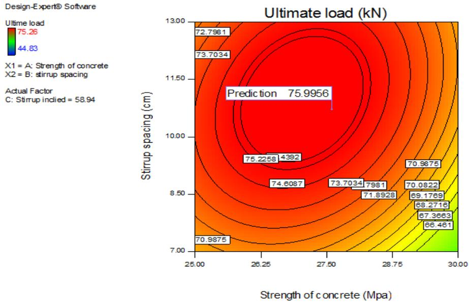
(a) Stirrup spacing = 10.71 cm, strngth concrete =27.60 MPa
