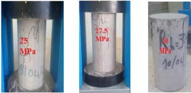
Figure 2. Strength compressive after compressive test
