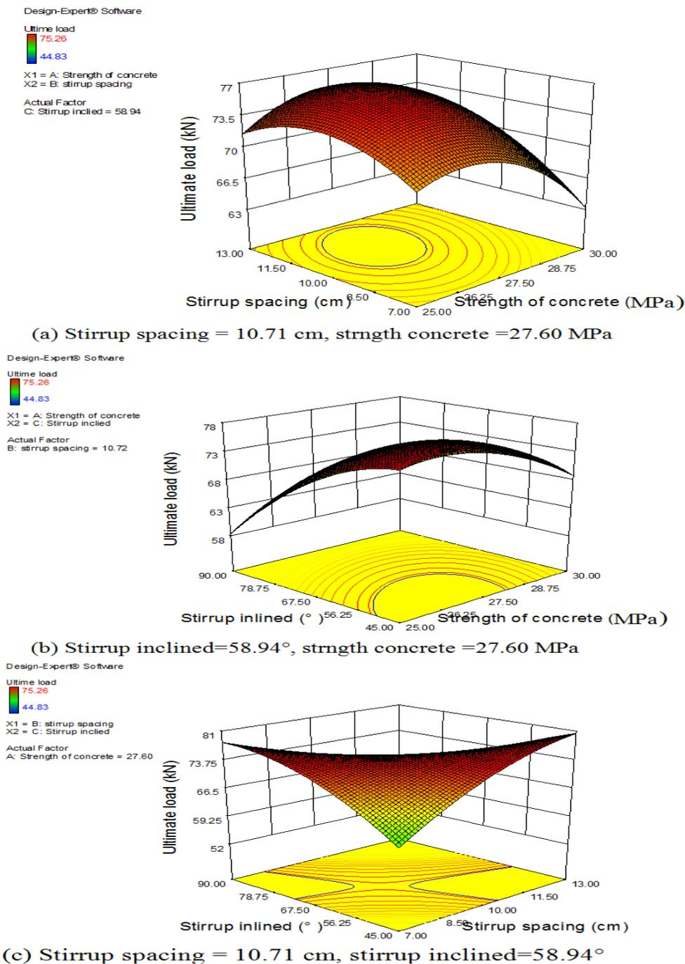
Figure 7. Response graphs for reinforced concrete beam
