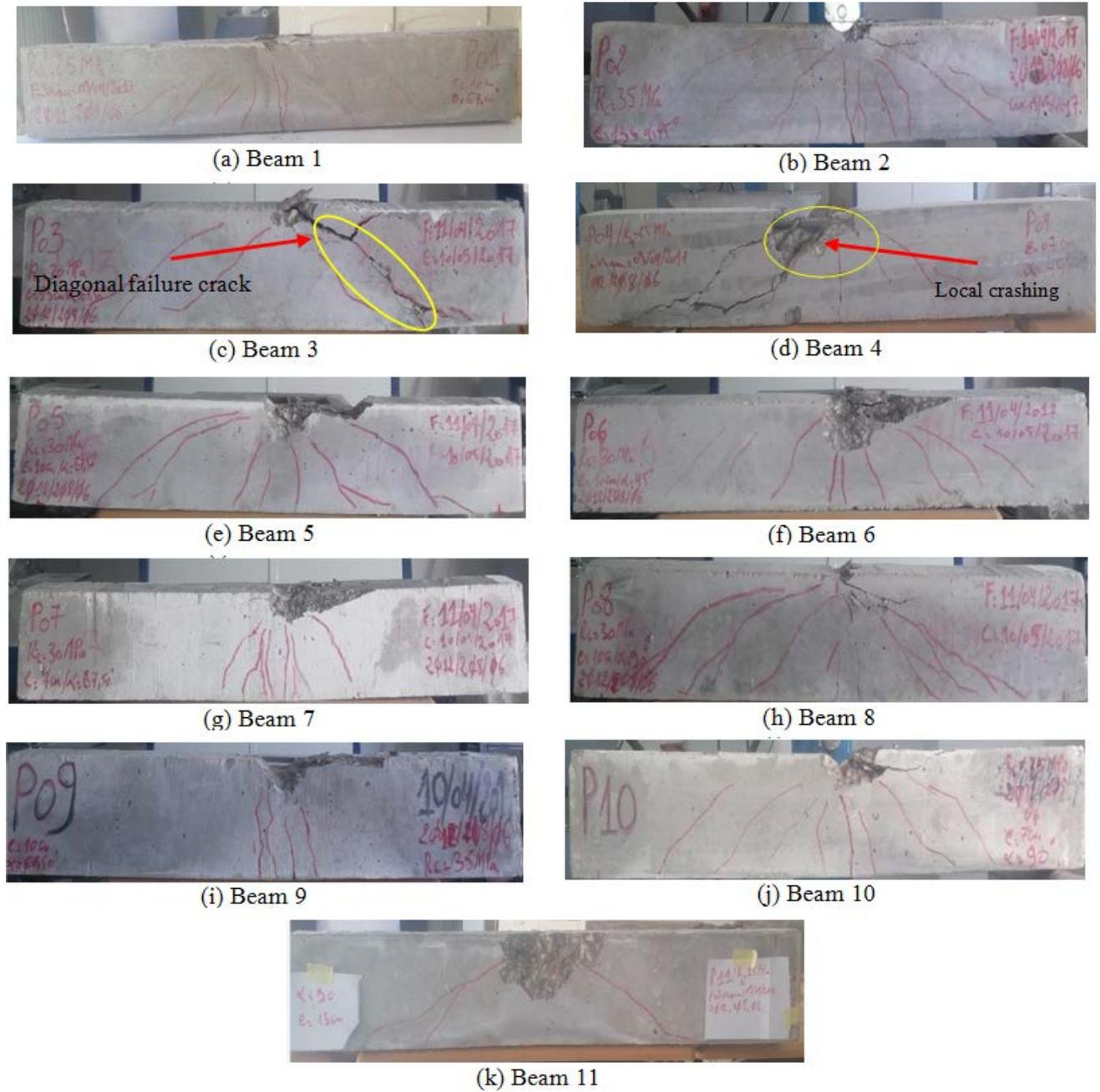
Figure 3. Crack patterns and failure modes of beams
