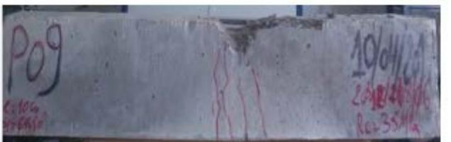
(f) Crushing the beams
