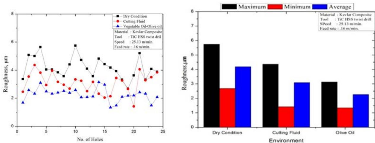
**Figure 5.** (a) Variation of holes' roughness ( $\mu\text{m}$ ) under different conditions. (b) The maximum, minimum and the average value of roughness under different conditions
