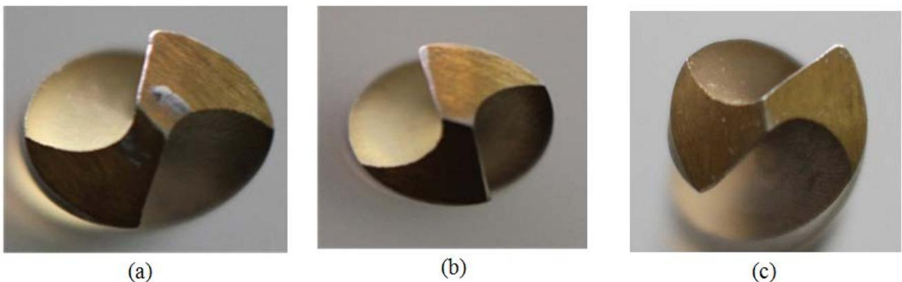
**Figure 6.** Photographic view of tool wear; (a) Dry condition (b) Cutting fluid (c) Vegetable oil (Olive oil)
