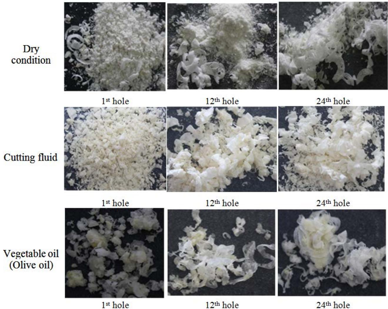
Figure 7. Photographic view of chips
