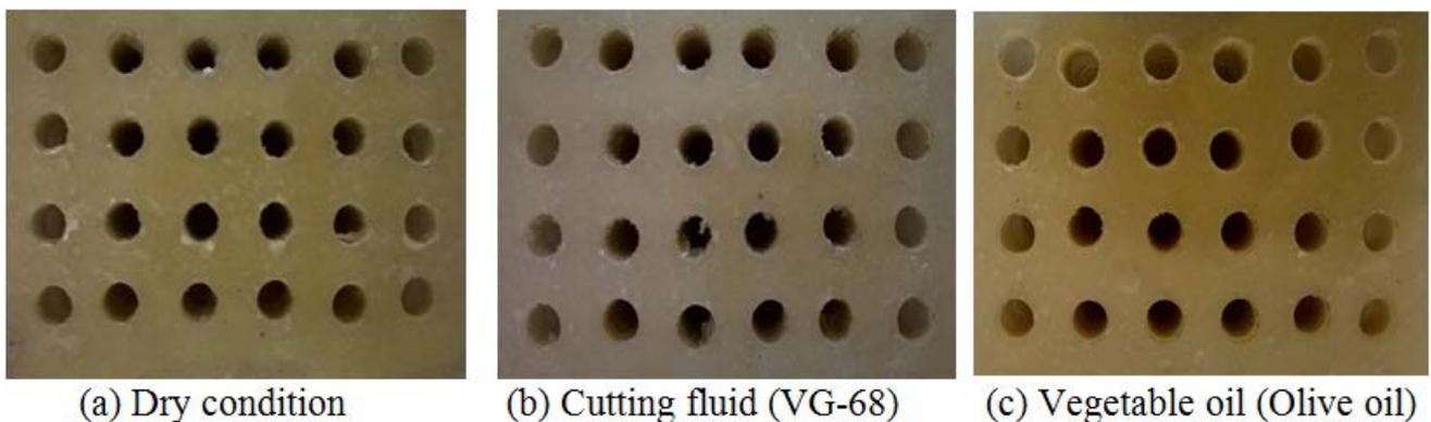
**Figure 2.** Photographic view of the drilled holes under different machining conditions**Table 2. The maximum, minimum and average diameter of holes at drill entry and exit under three different condition**
