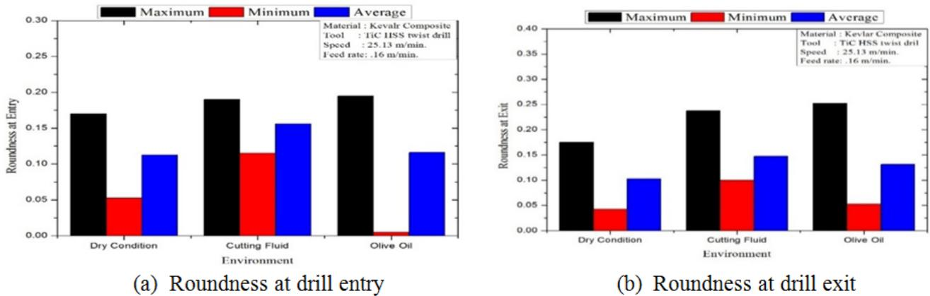
Figure 4. The maximum, minimum and the average diameter at drill entry (a) and drill exit (b) under different conditions
