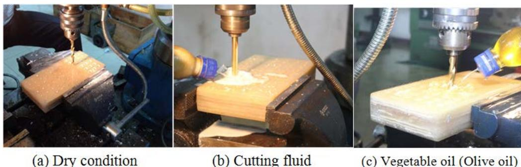
Figure 1. The photographic view of experimental investigation
