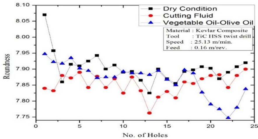
Figure 3. Roundness vs. No. of holes close to drill exit
