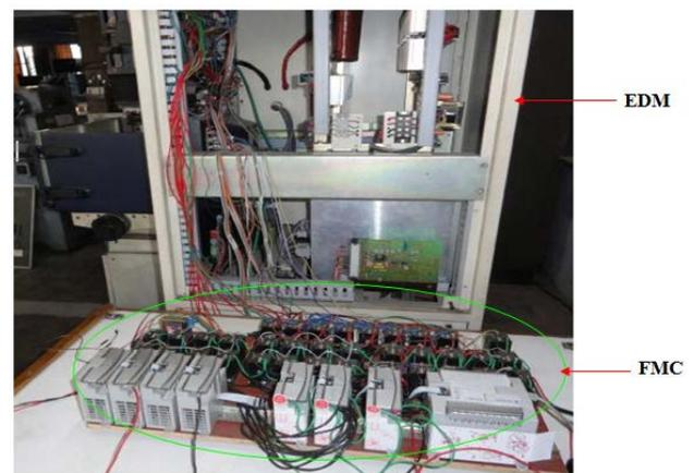
Figure 4. FMC Interface with die sinking EDM
