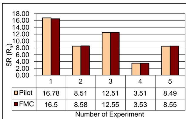
**Figure 5. Comparative analysis of surface roughness ( $R_a$ ) for AISI 52100**
