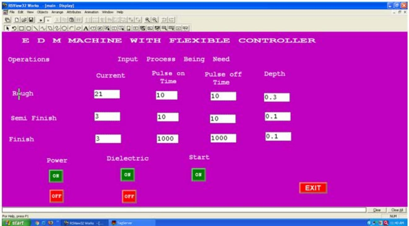
Figure 3. Flexible Machine Controller User Interface
