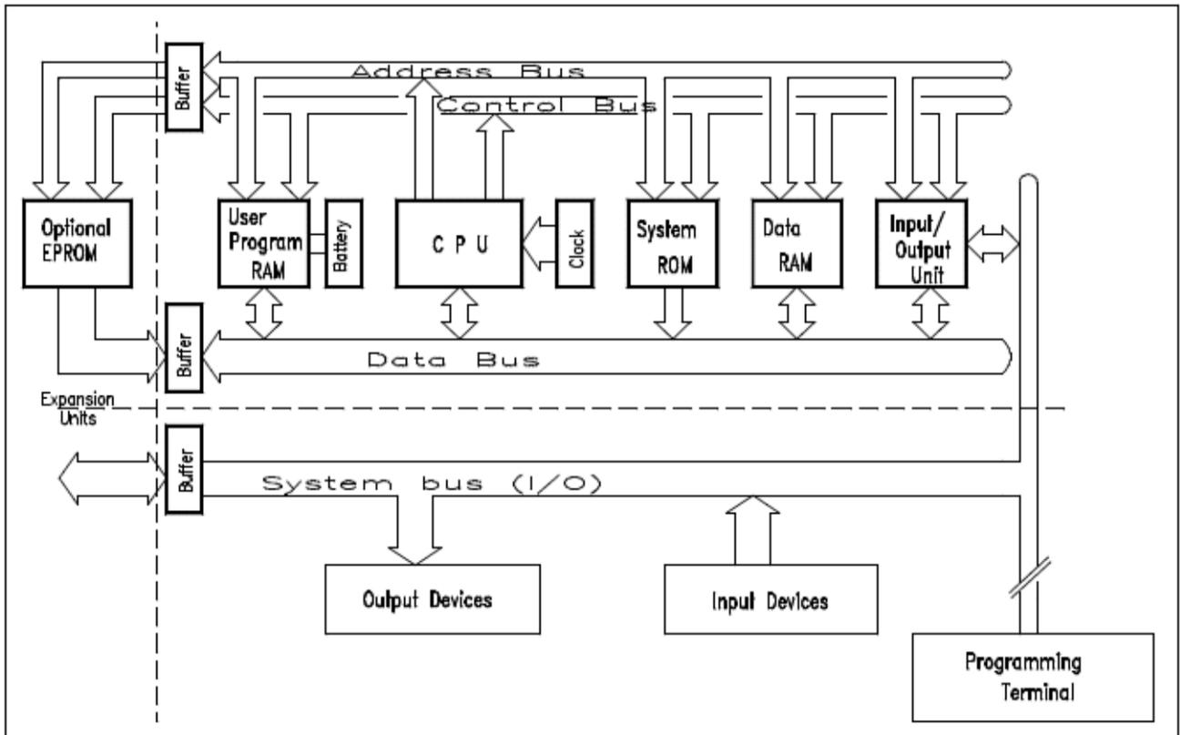
Figure 2. Block diagram of MicroLogix™ 1200 PLC CPU
